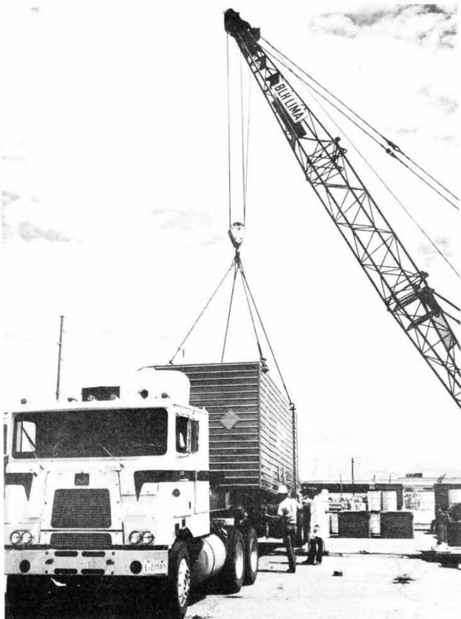
TRUPACT (TRansUranic PACKage Transporter) was designed for shipping defense nuclear wastes to storage sites or repositories such as WIPP (Waste Isolation Pilot Plant). Units would be carried by semi-trailer rigs or flatbed railcars.
