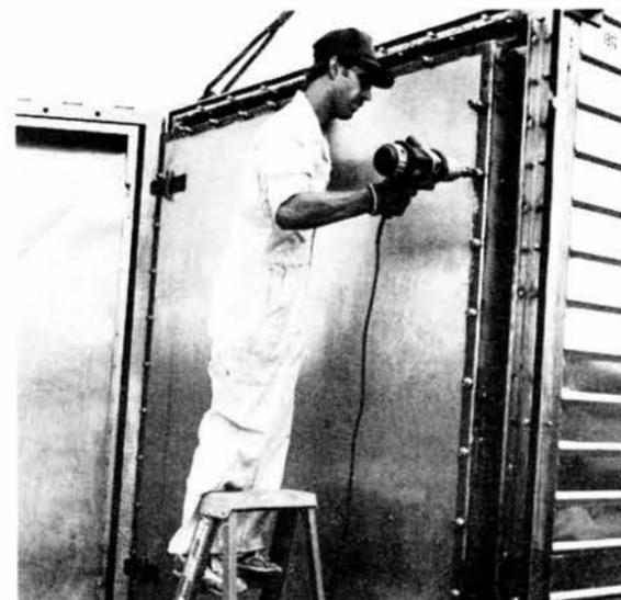
BOLTING the inner door is Dave Bronowski. Each TRUPACT is a steel box within a steel box with eight inches of rigid plastic foam, which serves as shock absorber and thermal barrier, separating the boxes.
