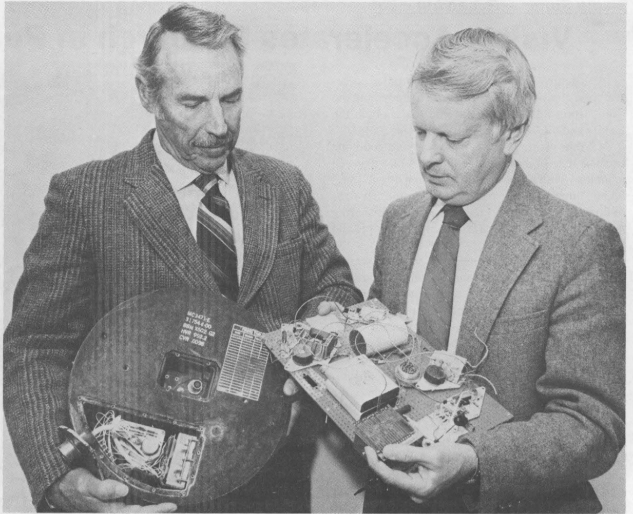
BEFORE AND AFTER — T. J. Williams (2361, right) holds a breadboard of the principal electronic modules and safety switches for the B83 firing set. Barney Barnette (2363) holds an encapsulated version of the same components, some of which are shown in the packaging cell at the bottom of the cylinder. Packaging ensures proper placement of components and protects them from severe or abnormal environments.
