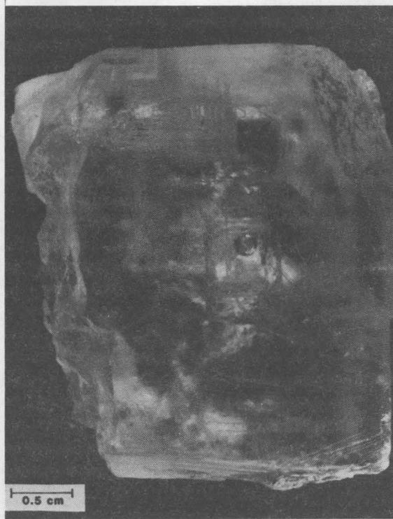
UNUSUALLY LARGE INCLUSION containing concentrated seawater (center, with bubble) appears in this sample of rock salt from the stratigraphic level of the WIPP facility 2150 ft. below the ground. Large inclusions, like this one measuring several millimeters on a side, permitted the brine to be extracted from individual inclusions and analyzed by standard wet chemical techniques.
