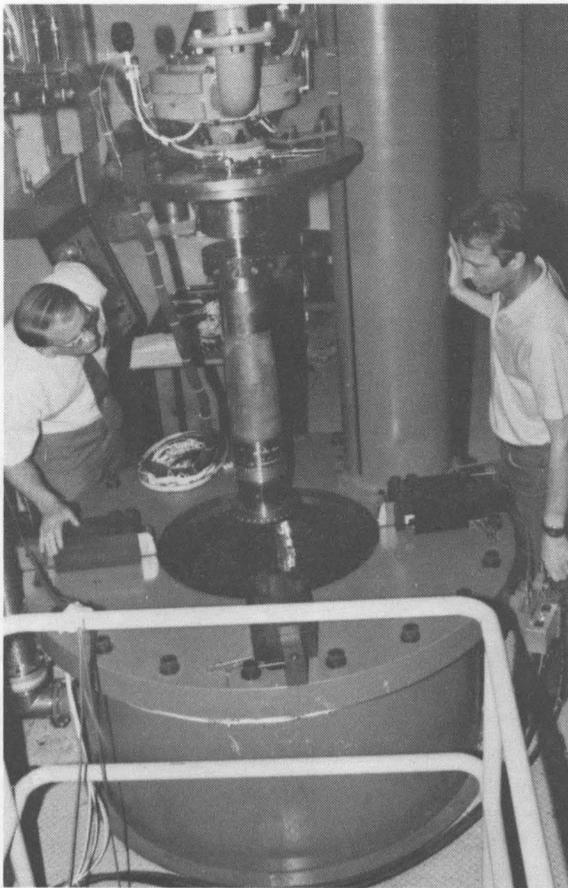
EXAMINING THE W82 test unit suspended on the shaft from the turbine above the six-foot deep containment tank are Pat Gildea (left) and Guy Prescott (both 8283). These test units are spun up to 18,000 rpm on the spin-test device.
