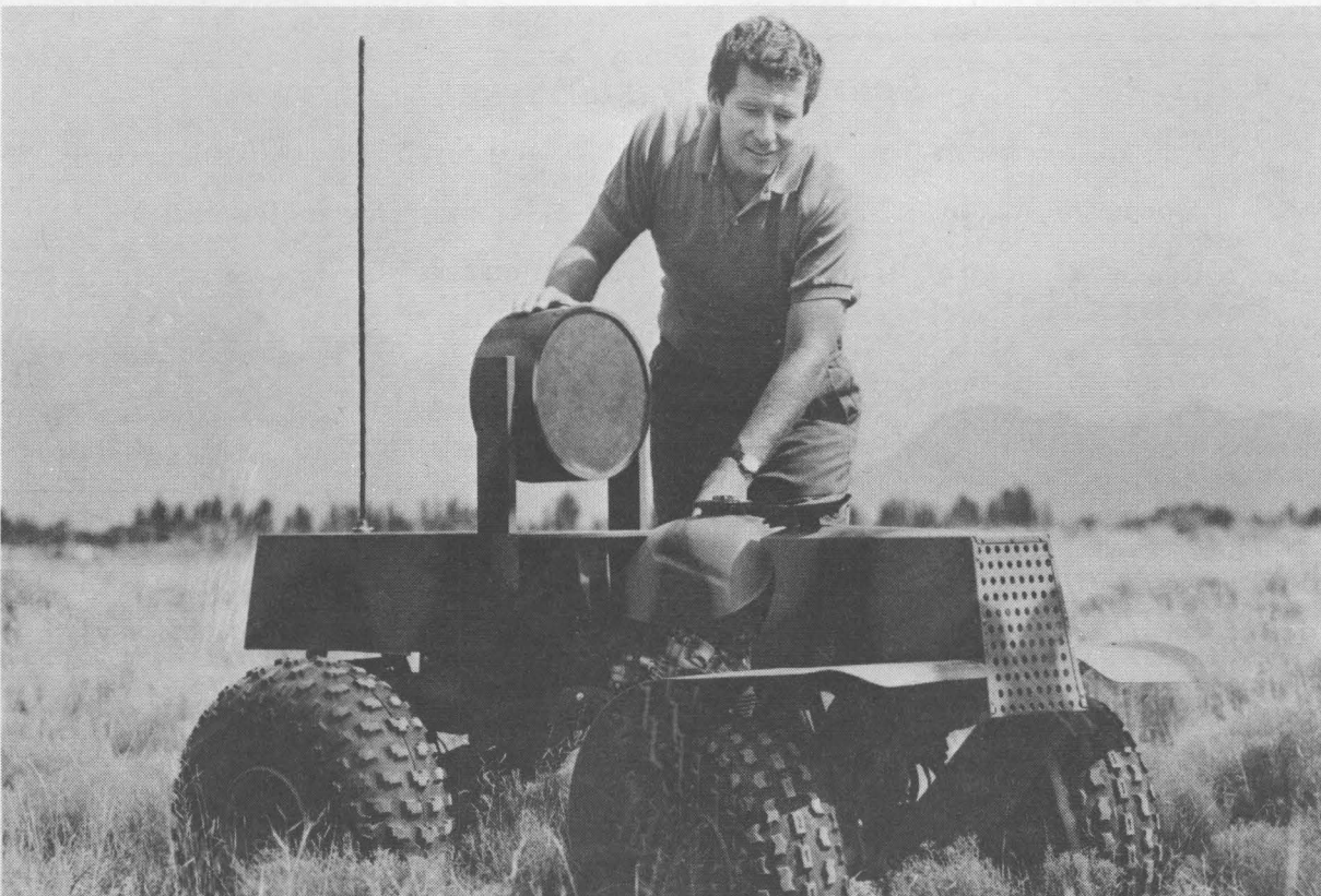
JAMES KELSEY (5267), whose division was responsible for overall Fire Ant system integration, displays a mock-up of the mean little critter. Round element at top, an explosively formed penetrator, is Fire Ant's warhead; during field test last fall, it destroyed a surplus tank.
