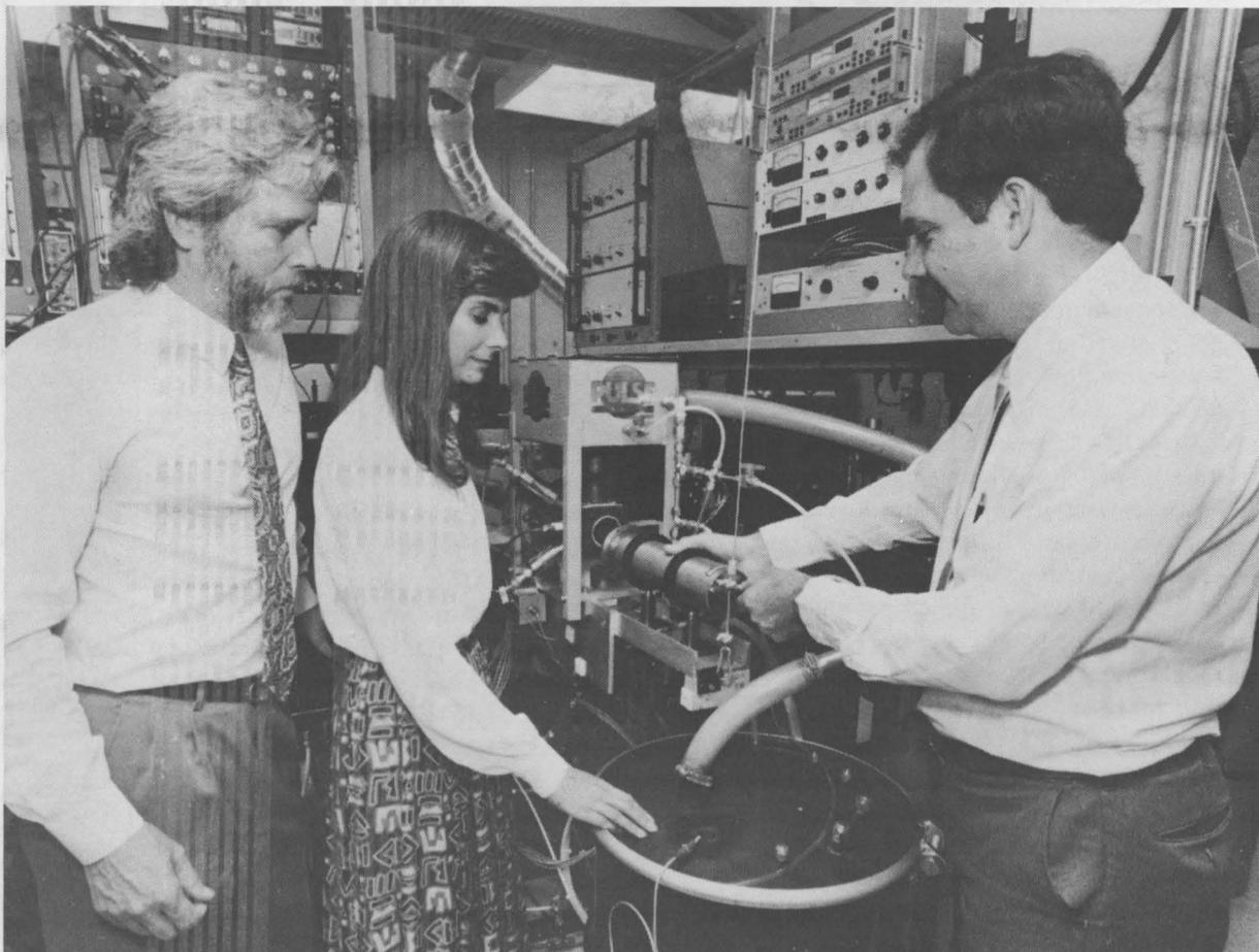
REASONS THAT PULSE COMBUSTORS are more efficient and less polluting than conventional combustion methods are becoming clearer due to research by Taz Bramlette (8364, left), Pam Barr (8363), and Jay Keller (8364). Jay adjusts photomultiplier tube used to reveal energy release in prototype Lennox pulse combustor hidden behind diagnostic equipment.
