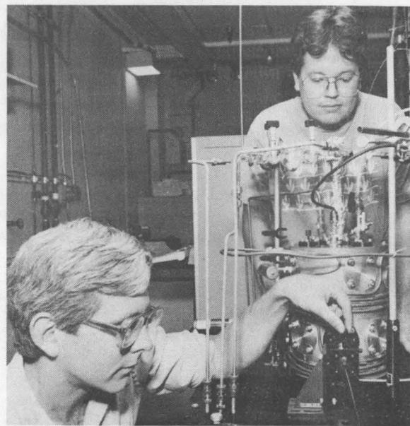
WHILE GEORGE WILKERSON (8353, right) looks on, Joe Durant (8353) aligns the fiber-optic output coupler of a laser photolysis/laser-induced fluorescence apparatus in CRF's Chemical Kinetics Lab. This and other research tools help scientists learn more about elementary gas phase reactions important for thorough analysis of the combustion process.
