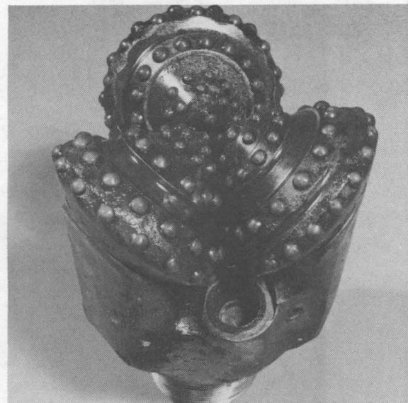
TYPICAL ROLLERCONE drill bit, basically unchanged since its invention in 1908 by Howard Hughes, Sr. Cones with tungsten inserts revolve as bit head rotates.
