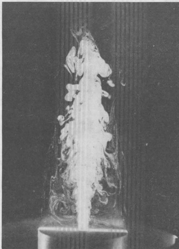
1/2-MILLIMETRE-THICK SHEET of laser light illuminates tiny nonburning alumina particles suspended in a flame. This helps CRF scientists learn more about gas flow in turbulent flames.
