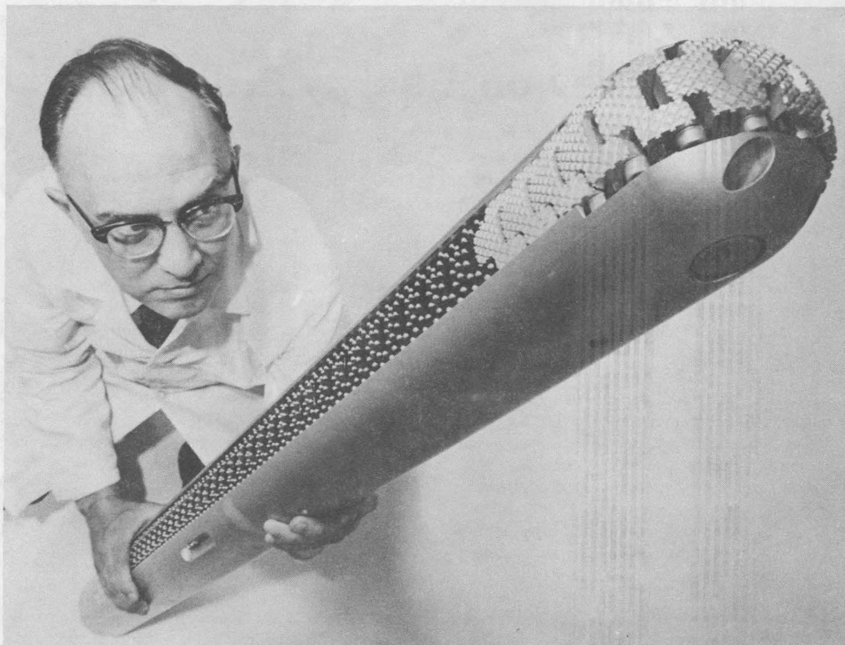
MODEL OF EXPERIMENTAL continuous chain bit, held by Dick Ashmore (ret.), shows cutting surface located on face of the chain, which advanced to bring new cutting surface into position. Despite promising initial test results, advanced development and testing were dropped.
