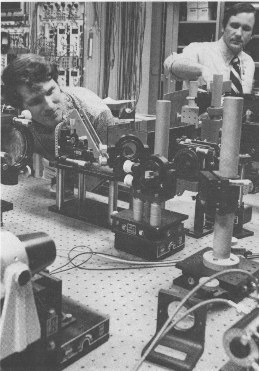
RETURN TO THE EARLY DAYS of CRF—vintage 1979—with Larry Rahn (DMTS, 8354) and Peter Mattern (8300) in a coherent anti-Stokes Raman spectroscopy (CARS) lab. Their work of about a decade ago led to techniques that significantly increased the detection capability of CARS, which remains a primary combustion research tool today for determining flame temperatures and major species concentrations.
