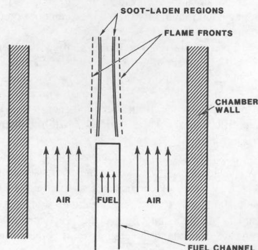
DIAGRAM of typical 2-D research flame used for soot and other studies at CRF.
