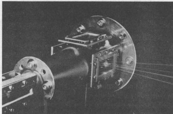
MULTIPLE LASER BEAMS enter combustion chamber of a research pulse combustor at CRF. Such laser-velocimetry experiments permit scientists to learn more about fuel/air mixing in the chamber and how actual combustion progresses.
