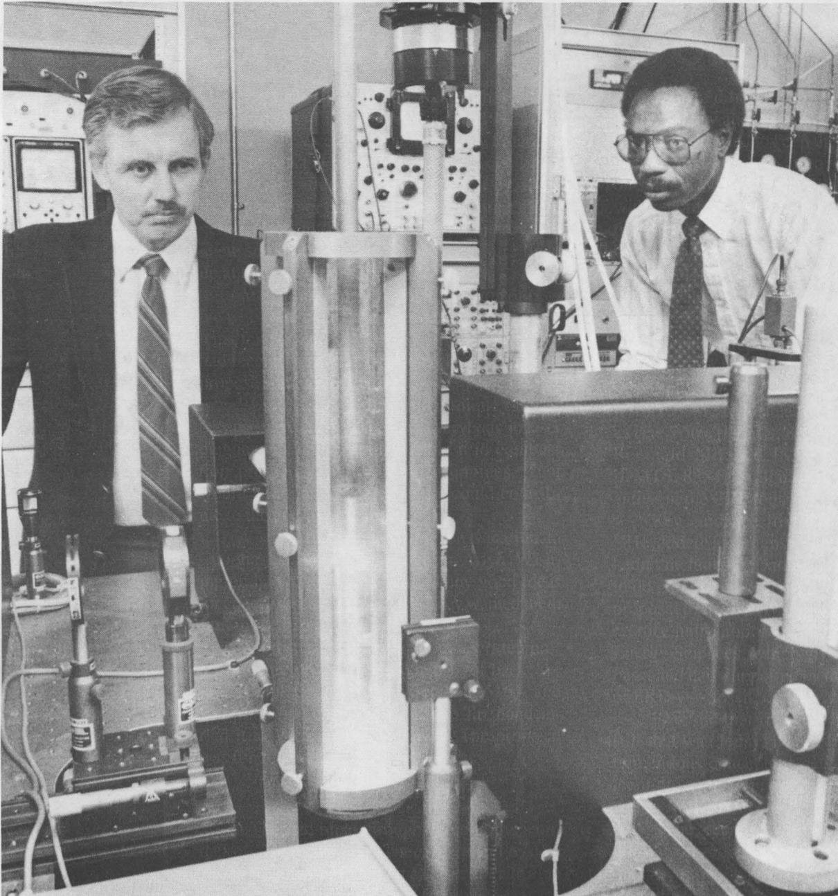
A KEY COMPONENT of CRF's Coal Char Combustion Lab is the laminar flow reactor that Don Hardesty (left) and Reginald Mitchell (both 8361) are watching. It burns pulverized coal in environments like those found in utility company boilers.
