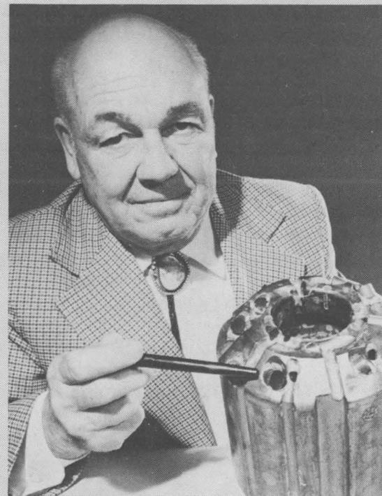
LENNY BAKER with an early PDC pressure-coring bit that he designed while at Sandia.
