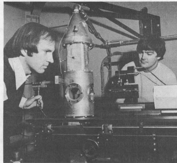
DAN HARTLEY (6000, left) and Pete Witze (DMTS, 8362) in 1975 setting up laser Doppler velocimeter on high pressure flame facility during early days of Sandia Livermore's combustion research.
