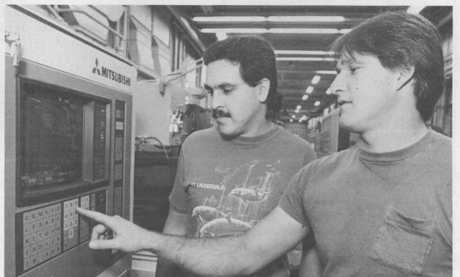
MACHINISTS Henry Apodaca (7481-5, left) and Gregg Jones (7482-2) use a numerically controlled wire-cut electrical discharge machine to cut work pieces.
