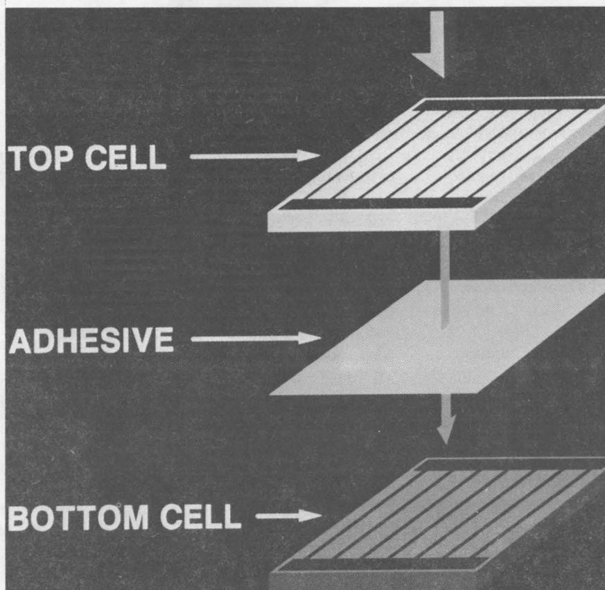
MECHANICALLY STACKED SOLAR CELL, shown in this diagram, is the result of work begun at Sandia in 1984. The top cell (gallium arsenide) captures solar energy from the high-energy (blue) part of the spectrum, while the bottom cell (silicon) absorbs energy from the low-energy (red) portion. The new composite cell has attained the highest-ever PV conversion efficiency — 31 percent — in lab tests.
