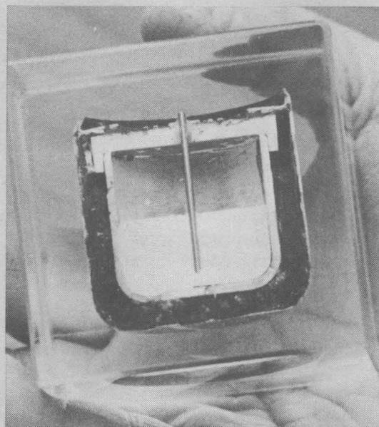
CUTAWAY of a typical sodium/sulfur rechargeable battery imbedded in plastic. Dark U-shaped section is sulfur electrode; white material in center is sodium electrode that surrounds metallic rod terminal. Thin gray "U" between electrodes is beta-alumina electrolyte/separator.
