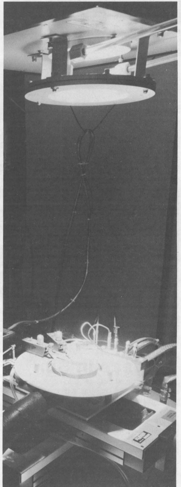
LENS-CELL TESTER is used by Labs researchers to characterize lens/cell combinations for possible use in PV concentrator modules.
