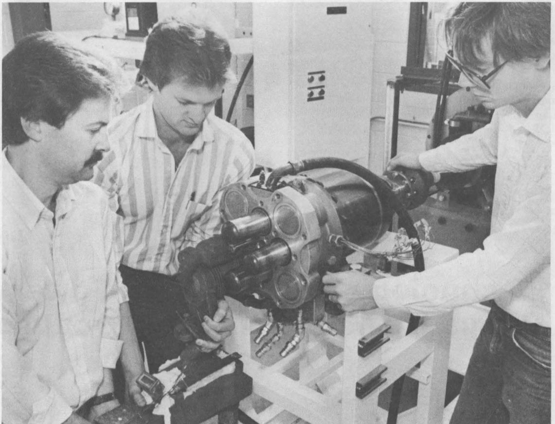
KEVIN LINKER (left, 6227), Scott Rawlinson (6222), and Doug Adkins (6227) attach a heat pipe to one of the four cylinder-head heaters of the new STM Stirling engine to be tested soon at Sandia.
