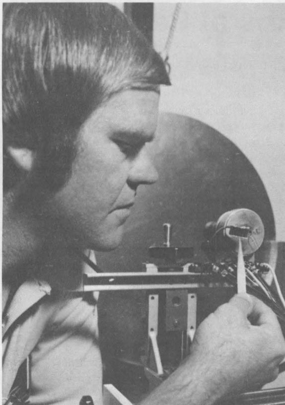
MID-70s-VINTAGE solar cell being readied for high-artificial-illumination tests aimed at reducing solar cell size. That's Ed Burgess (now 400), one of Sandia's early-day solar researchers.
