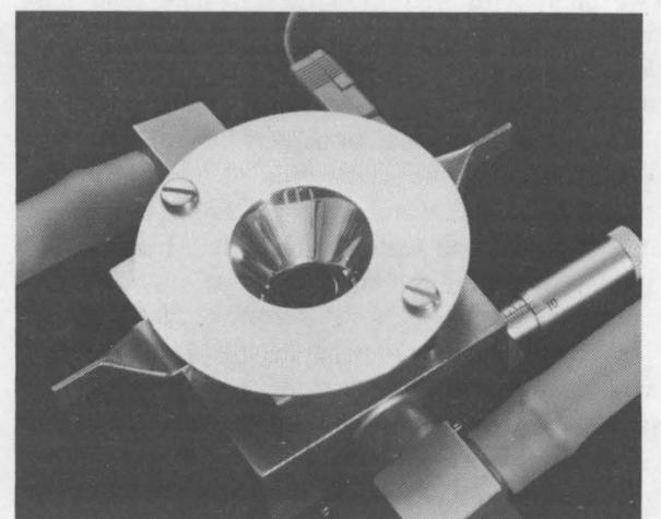
DETAIL OF PV SYSTEM developed in the early 80s, showing reflective brass cone mounted on solar cell housing. Cone's purpose is to help increase solar cell module efficiency.
