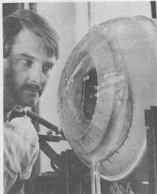
DIRECT CATALYTIC ABSORPTION RECEIVER, designed by Rich Diver (6227), uses concentrated solar energy to destroy hazardous wastes such as those created during microelectronics fabrication. During optimum sunlight, receiver of this size could chemically transform about two litres of waste every hour.
