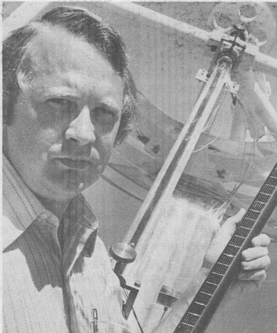
DURING EARLY DAYS of solar R&D, Don Schueler (6220) and others were interested in determining feasibility of integrated solar collectors to produce both electricity and heat. Here, Don holds equipment for such a system — a special receiver tube with silicon solar cells mounted on its surface.
