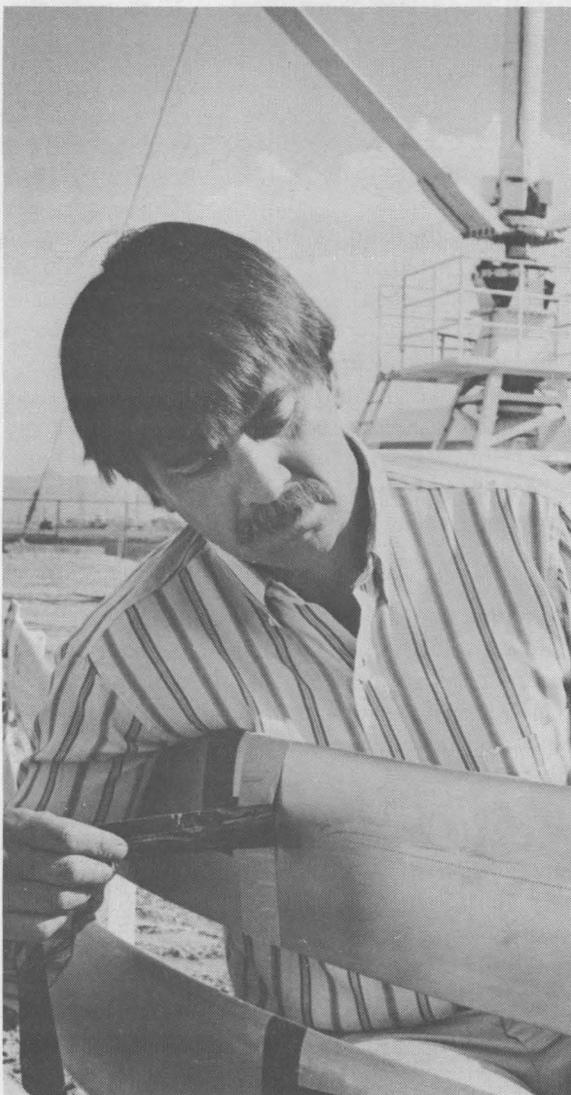
PAUL KLIMAS (6227) inspects some matchstick-diameter holes drilled in VAWT blades. The holes are key to a patented spoiler system that allows VAWTs to operate more efficiently in extremely high winds. Spoiler, patented in names of Paul, Emil Kadlec (DMTS, 9122), and Jack Cyrus (9122), limits torque produced by whirling blades during peak winds.
