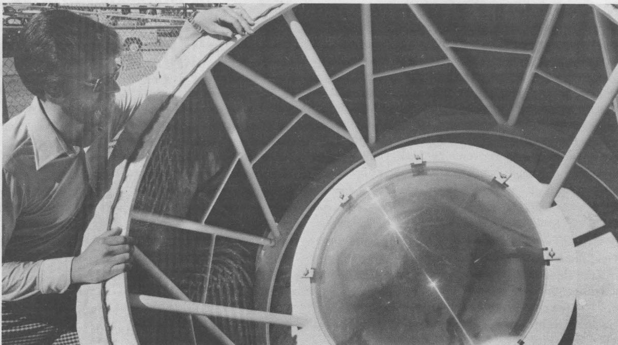
FRESNEL LENS on a two-axis tracking device developed in the mid-70's by Gene Hammons (1144) for measuring efficiency of solar cells. Gene received a patent for the tracker.
