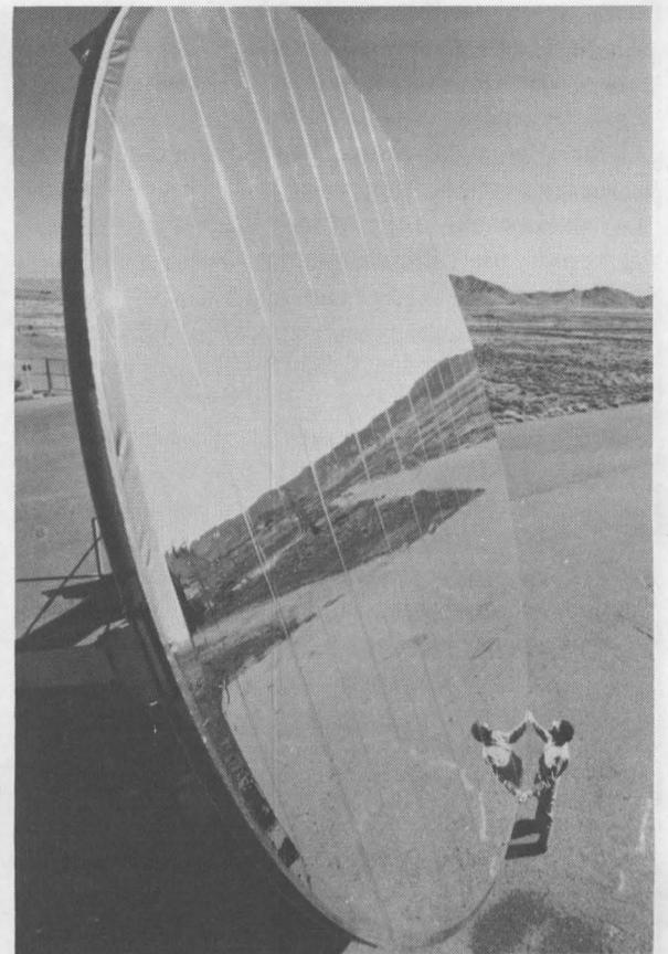
DAN ALPERT (6226) checks surface of a stretched-membrane heliostat tested here. Work is under way on design of a new stretched-membrane heliostat, using lessons learned from testing this and other prototypes.
