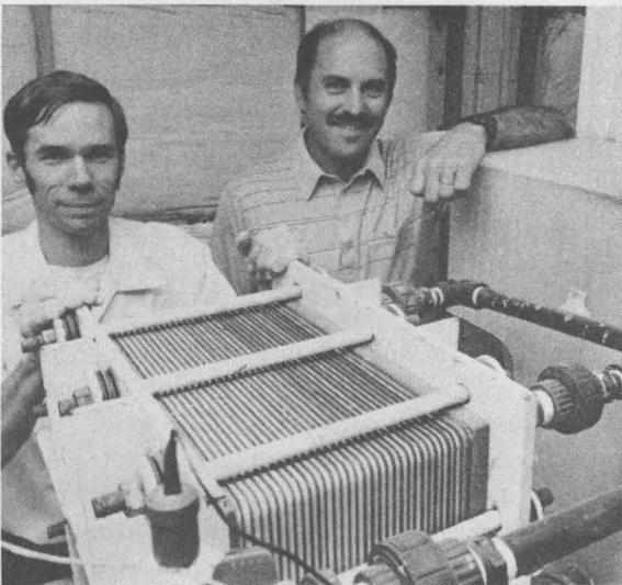
BLDG. 833 IS HOME for a prototype zinc/bromine load-leveling battery, which has 30 cells and a 125-amp-hr. capacity. Paul Butler (left) and Jeff Braithwaite (both 2525) stand behind the battery, which requires external tanks to hold liquid electrolyte that flows through cells during operation. Paul is next to cell array; Jeff leans against one of two electrolyte storage tanks.
