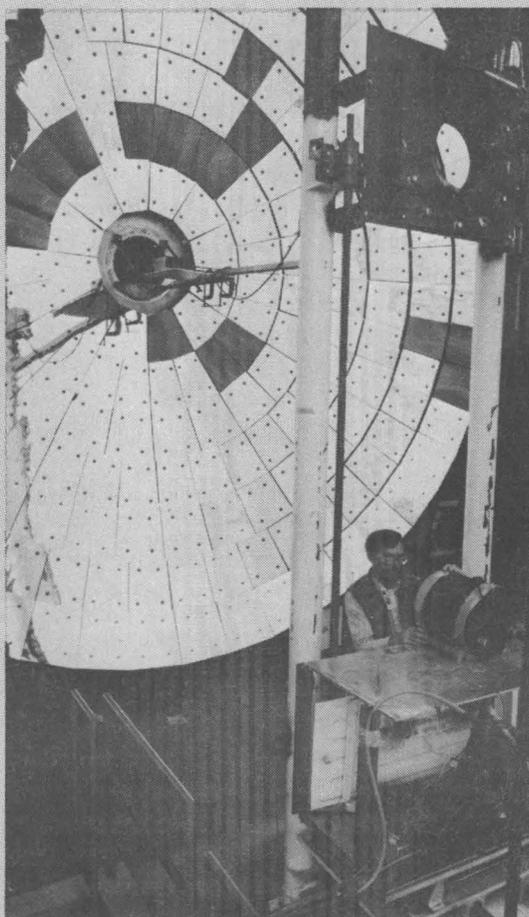
BOB EDGAR (6222) adjusts calorimeter before calibration test at Sandia's solar furnace. Test object is placed at focal point of furnace's 22-ft.-diam. parabolic dish behind Bob.
