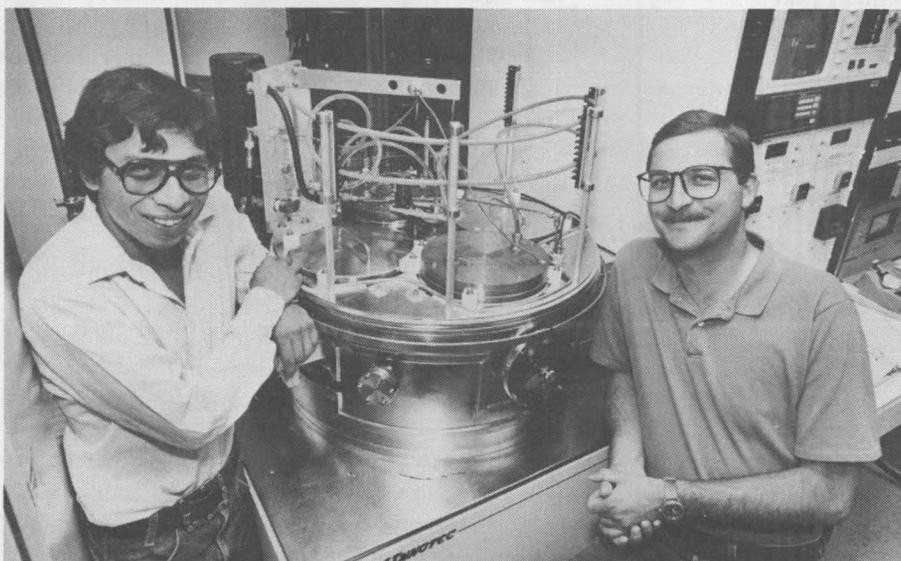
TANTALUM NITRIDE SPUTTERING SYSTEM between materials tradesmen Frank Lucero (left) and Dave Jones (both 7411-1) is used for metal deposition on substrates.
