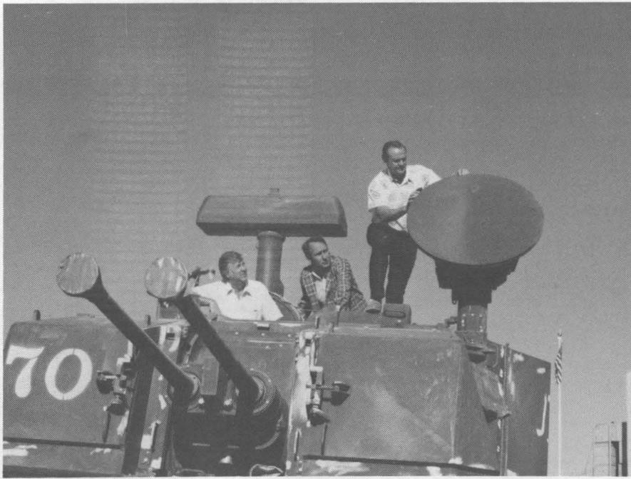
RADAR SYSTEM on one of the York guns is checked at the Tonopah Test Range by (from left) Carl Smith (7174 supervisor), Jerry McCorkle (7174), and TTR manager Ron Bentley (7170). The sophisticated radar system is the same type used on the advanced F-16 fighter aircraft — the Fighting Falcon. The round unit that Ron is checking is a targeting radar; the rectangular unit is a surveillance radar. One of the uses planned for TTR's Yorks is mobile radar tracking of targets.
