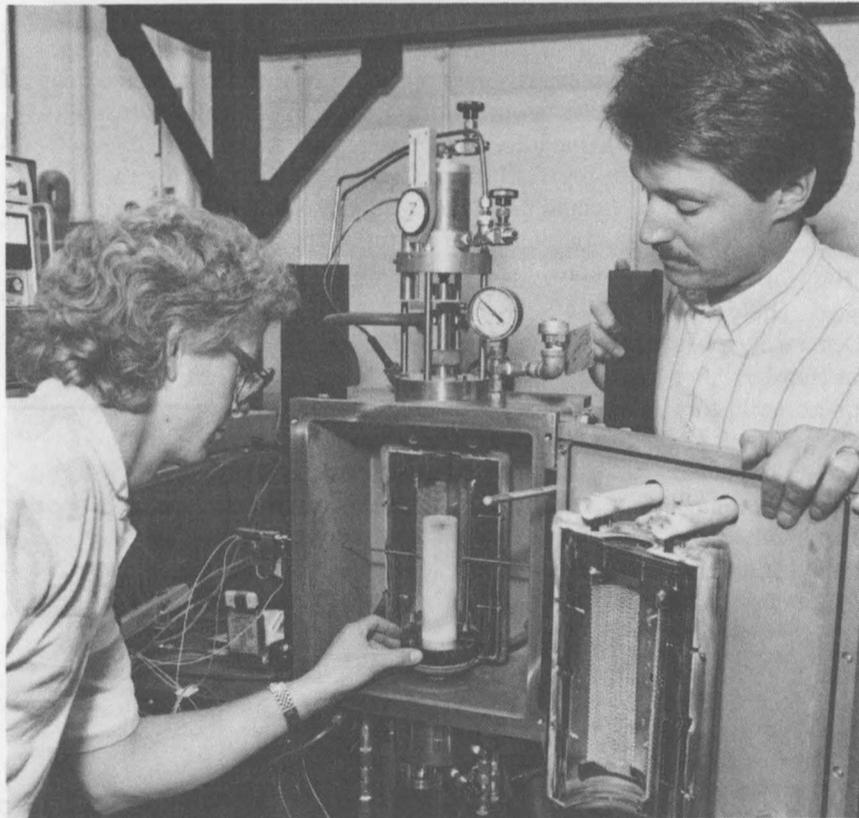
THE HEAT IS ON — or soon will be — for boride samples inside this furnace. Stuart Van Deusen (left) and Terry Ase-lage (both 1842) are working to produce materials for research that could lead to high-temperature semiconductors; the furnace melts its contents at about 1800°C and lets single crystals form by cooling slowly to about 1000°.
