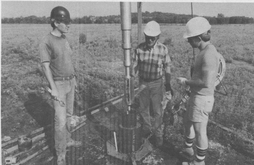
**GEOPHYSICAL RESEARCH SPECIALISTS** (from left) Sandy Ballard, Gerald Reynolds, and Greg Elbring (all 6231) prepare to lower the downhole seismic source into a drill hole during field tests at Amoco Production Company's test site near Tulsa, Okla., earlier this year.
