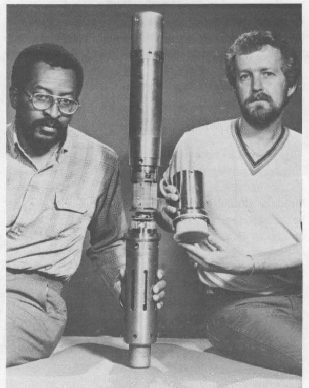
FRED HEARD (left, now 9234) and Tom Bauman (now 9127) teamed for development of the geothermal high-temperature, high-pressure acoustic borehole televiewer. Fred holds acoustic sensor assembly — motor, rotating transformer, magnetometer, and transducer. Tom displays a magnetometer pressure housing section.
