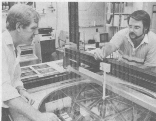
TOM BICKEL (left) and Bruce Engler (both 6258) check settings on the geoelectric simulation facility. Gold-coated copper triangles making up GSF's fluid-filled basin are computer-controlled to vary resistance settings, matching field conditions.
