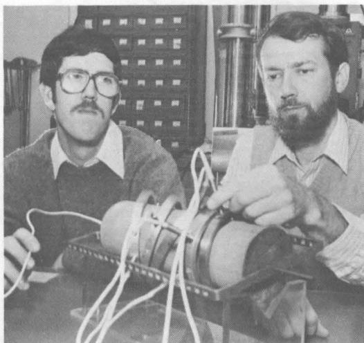
ANELASTIC STRAIN RECOVERY technique is possible because of this patented tool designed by David Holcomb (right) and Mike McNamee (both 6232). It can detect core movements (strain relaxations) as small as one-millionth of an inch.
