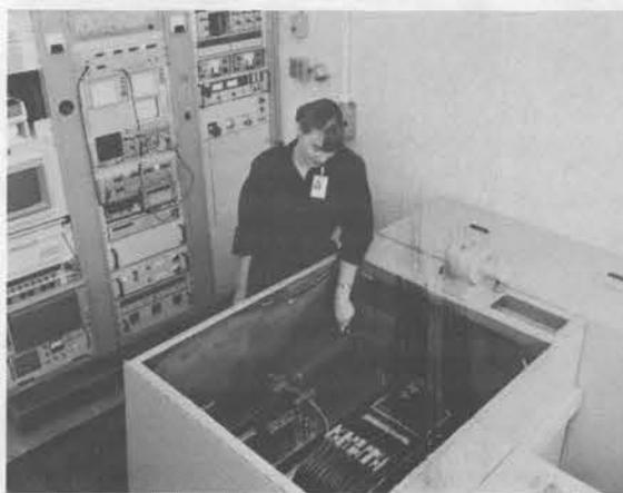
HIGH-VOLTAGE PULSE GENERATOR in Primary Standards Lab consists of three subsystems: the test tank (shown with top cover open), which contains the high-voltage pulse transformer and the voltage standards to be calibrated; the oil storage tank (right rear), where oil is stored between calibrations; and the instrumentation rack.
