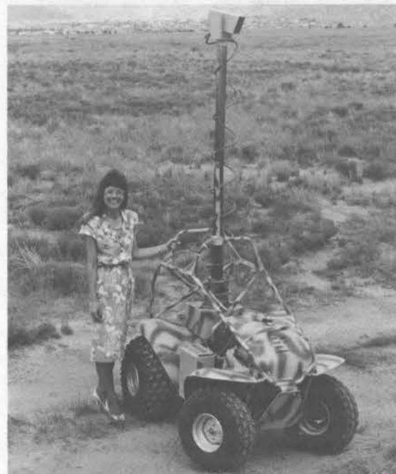
"DIXIE," a mobile reconnaissance vehicle that's operated remotely from a base station some distance away, is displayed by Connie Vanderburg of Nuclear Security Systems 5200. TV camera is mounted on the extendable mast.
