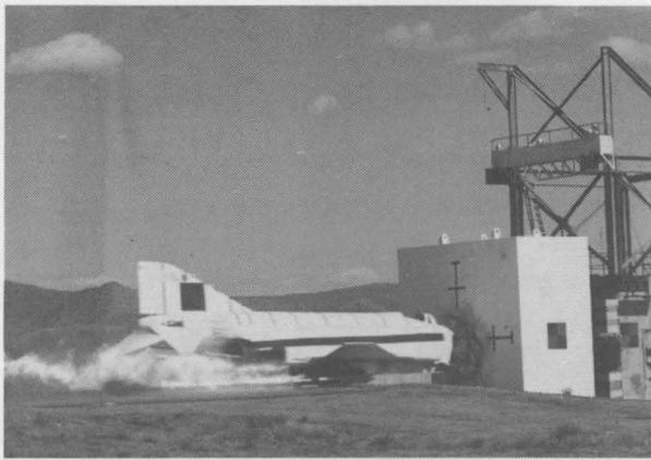
GOING, GOING, GONE — Sequence shows rocket sled test of F-4 Phantom jet aircraft as it slams into a one-million-pound block of concrete. The first-of-its-kind test was designed to help researchers estimate the effect of an aircraft crashing
