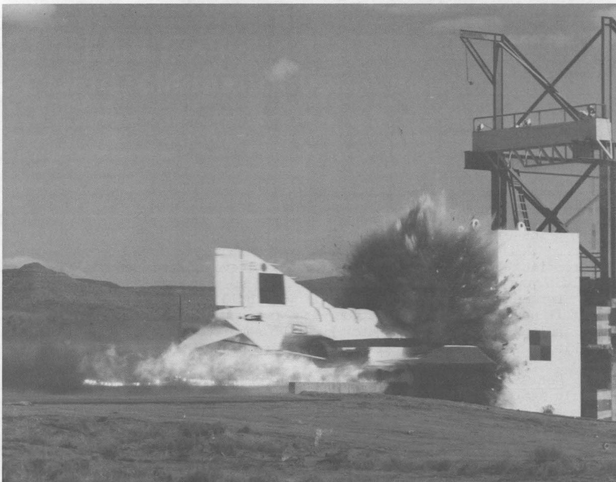
THIS FULL-SCALE IMPACT TEST at Sandia demolished an F-4 Phantom instantly. The test was funded by the Muto Institute of Structural Mechanics, Inc. (Tokyo) and performed here on the Labs' 2000-ft.-long rocket sled track under terms of a joint US-Japanese agreement for cooperation on nuclear safety engineering and research. See additional photos of the test sequence on page four. (Photo courtesy of Photometrics and Optical Development Div. 7556)
