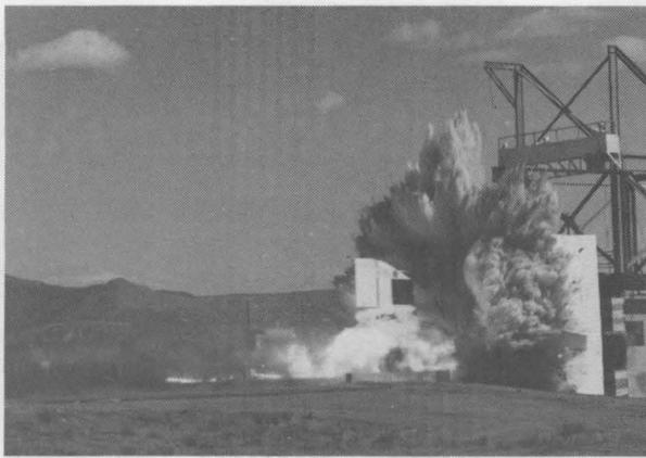
directly into a nuclear power-plant structure. A 70-mm framing camera running at 125 photos per second froze the action. (Photos courtesy of Photometrics and Optical Development Div. 7556)
