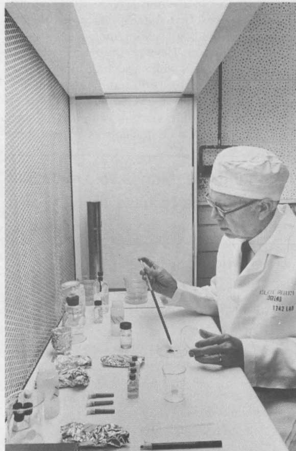
EARLY LAMINAR AIR FLOW WORK STATION: Filtered air passes from filters in the gridded wall at left and flows over the work area.
