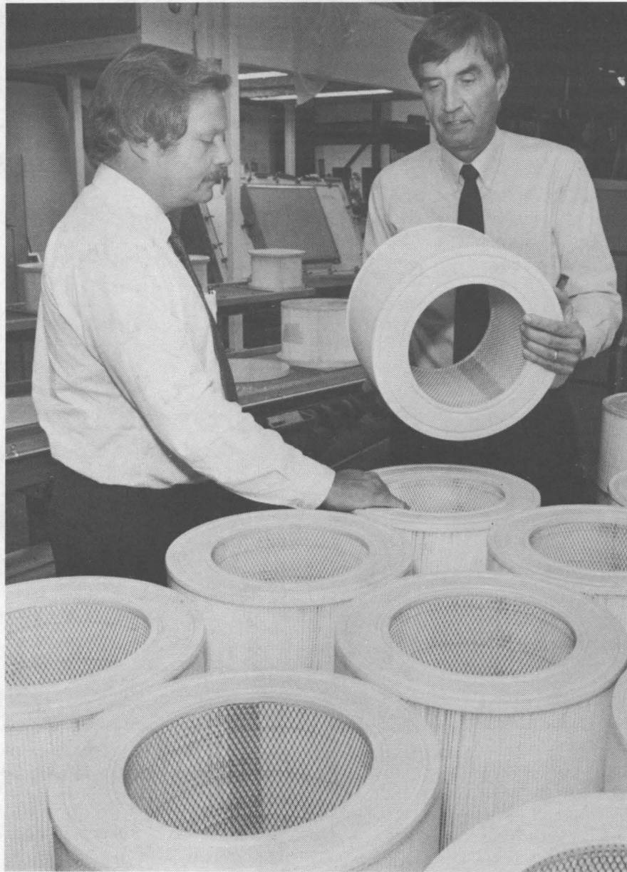
LAMINAR FLOW AIR FILTERS are inspected by David Schlegel (left) and Skip Erickson at the Envirco Division of Environmental Air Control Inc. (EACI). Schlegel is general manager of Envirco and executive vice-president of EACI. Erickson is Envirco Company Controller. The filters are just one of an extensive line of laminar flow contamination control equipment built in the Albuquerque plant, which employs about 78 people. Most of the company's products are based on the clean room concept invented by retired Sandian Willis Whitfield.
