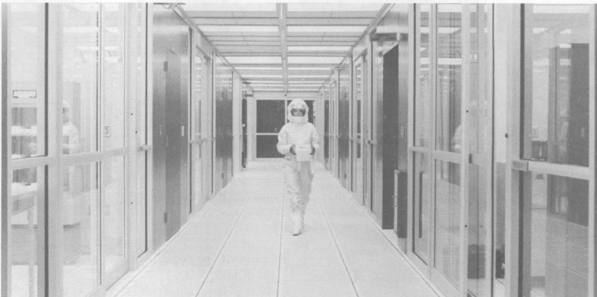
CLEAN ROOMS are used throughout Sandia today. Here, April Howard (2131), wearing a special clean-room suit, transports a set of silicon wafers down the aisle between clean-room bays in the Microelectronics Development Laboratory. The muted lighting in the photo is from safelights that protect unexposed wafers.
