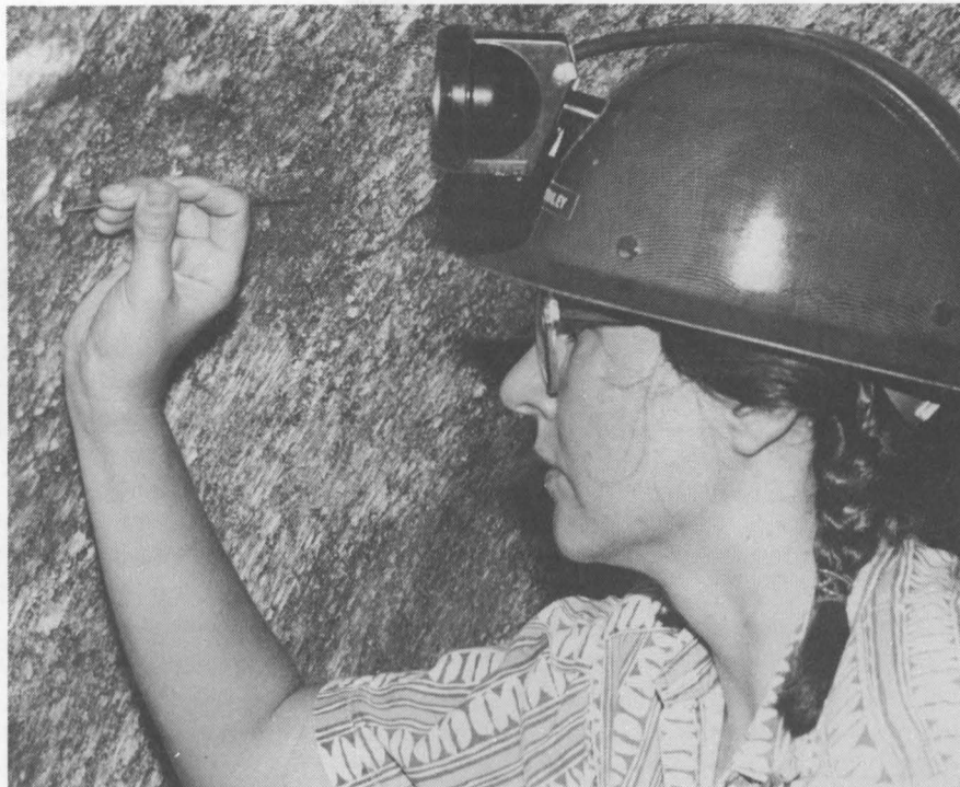
SAMPLE TAKING: Sharon Finley (6344) uses a capillary tube to capture a brine sample from a freshly mined surface. Such samples and analyses have helped scientists understand the limited fluid movement that occurs within the Salado Formation.
