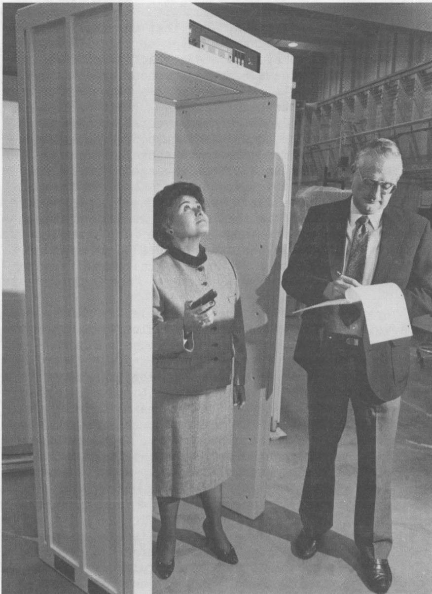
HOLDING A GUN — but purely for calibration — Terri Olascoaga (5248) checks whether a metal detector is responding to the weapon, as Don Gould (5248) makes notes. Detectors used in the airport-security project at Baltimore-Washington International will be calibrated for triggering by test weapons that the Federal Aviation Administration plans to use as a standard in the future — weapons that are smaller and harder to detect than those currently used for setting the detectors.
