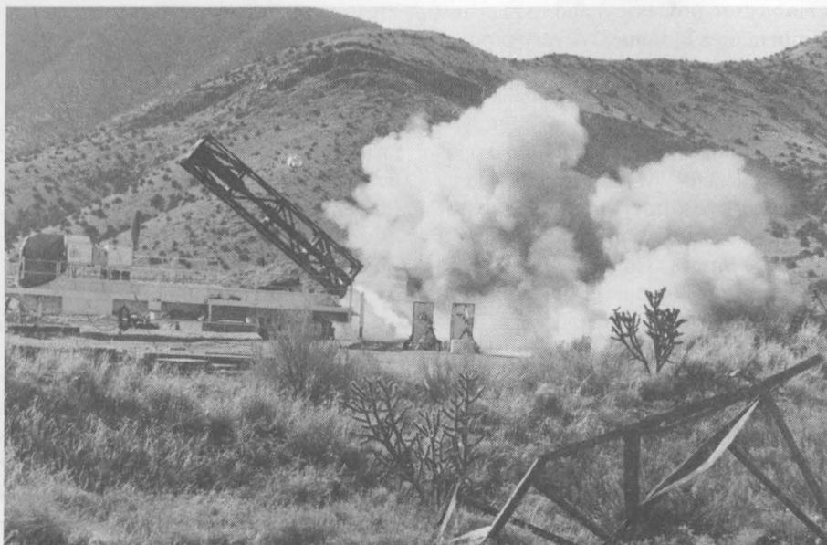
SANDIA-DEVELOPED PORTABLE GAS GUN was used for stability assessment tests on the Navy's Advanced Bomb Family penetrator. Here, a 100-lb. projectile slams into a 6-in.-thick reinforced concrete slab at 700 ft./sec.
