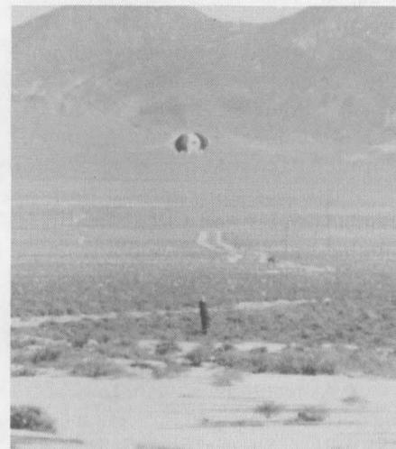
**PARACHUTE RECOVERY SYSTEM** to soft-recover artillery projectiles fired from 155mm howitzers has demonstrated increased reliability, compared to its predecessor, in all 15 of its tests to date. The test shown here was at Tonopah Test Range.
