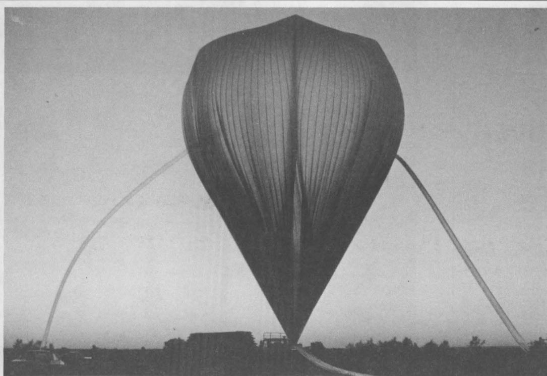
SPACE BALLOON, ready for launch on a previous mission, carries a gamma-ray instrument for observing neutron stars, supernova remnants, and black holes.
