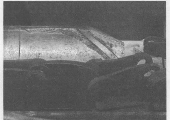
**DISTORTED RAMMER LINKS** inside gouged spanner tray. Different-sized links — some 4.4 inches long and some 4.8 inches — left identifiable marks in the tray as the explosion blew them sideways and backwards. (US Navy photo)
