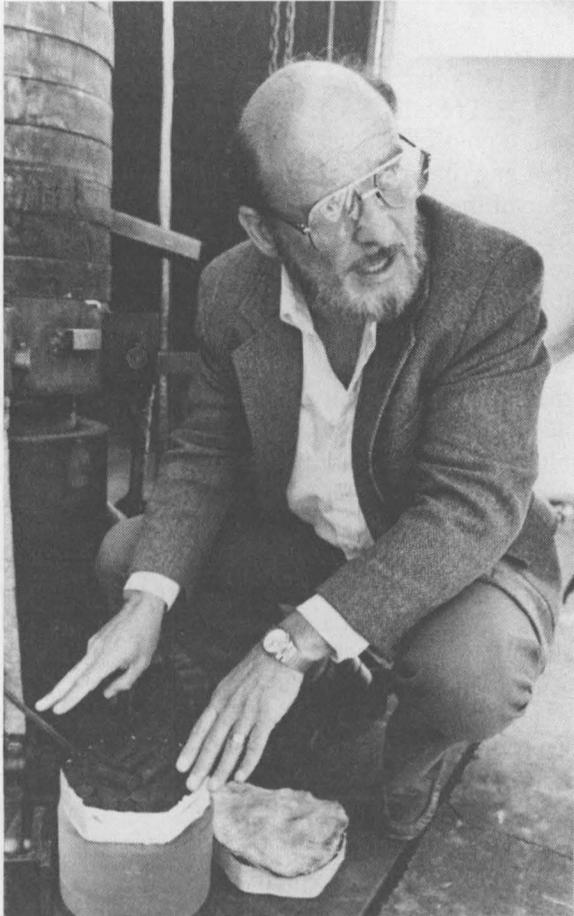
PAUL COOPER (DMTS, 9333) explains the half-scale test apparatus used for impact-ignition experiments. Small black cylinders near his left hand are propellant pellets, which are arranged on a large plastic cylinder that simulates the mechanical properties of more layers of pellets.
