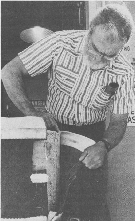
KARL SCHULER (DMTS, 1522) looks at a propellant bag of the type involved in the *Iowa* incident. The dark material is a wear-saving cover; the lighter, laced bag inside is the silk propellant bag.
