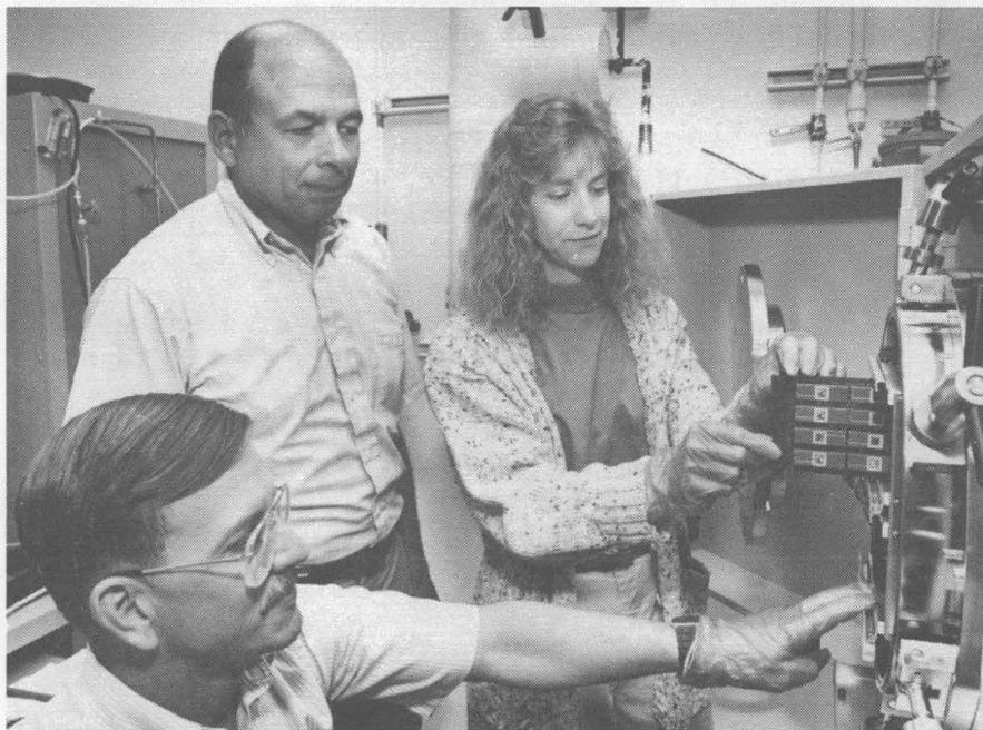
JIM SWEET (2134, center), designer of the assembly test chip, watches colleagues Dave Peterson and Melanie Tuck (both 2134) put chips into a highly accelerated stress-test chamber, where the chips will be subjected to temperature and humidity testing to evaluate the moisture resistance of the packaging.
