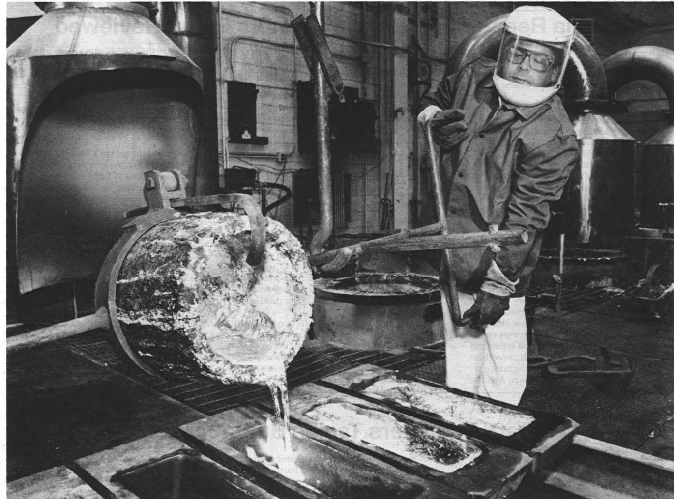
STANDING BACK a respectable distance, tradesman Gary Gallegos guides a system of bars and cranes to tip a crucible of molten aluminum over a waiting ingot mold of steel. The aluminum ingots are stored for future use.
