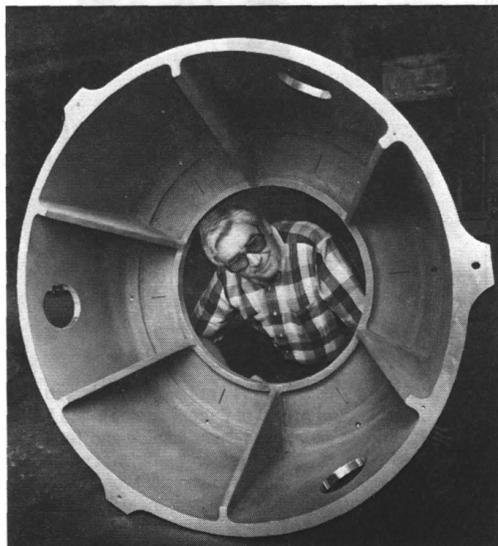
WAYNE CYRUS examines an aluminum alloy casting that will be used for a mobile camera base to be mounted on a trailer at the Tonopah Test Range in Nevada.
