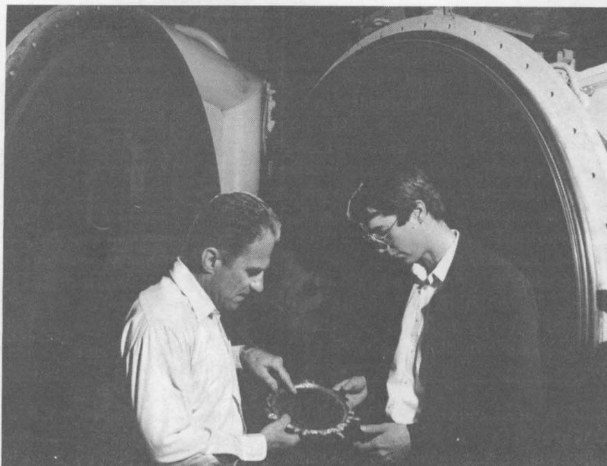
FRANK ZANNER (DMTS, 1833, left) and Phil Sackinger (1511) discuss the solidification of a titanium ingot. They're standing in front of a vacuum induction furnace used for metallurgical research.
