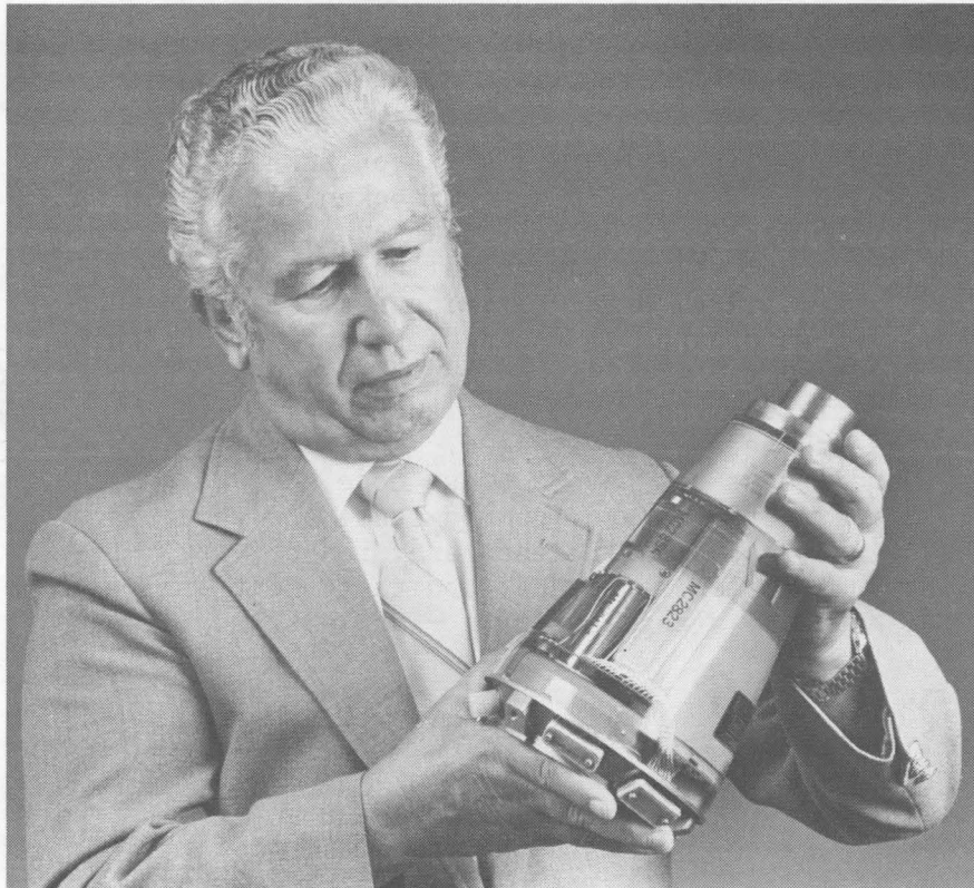
JOHN SOUZA (5154) is the only Sandian who was on the MC2912 arming, fuzing, and firing system program in the beginning and was still with it at the end. Here, he holds a "show-and-tell" display unit of the football-sized AF&F system; the transparent potting material encasing the unit allows various components to be viewed.
