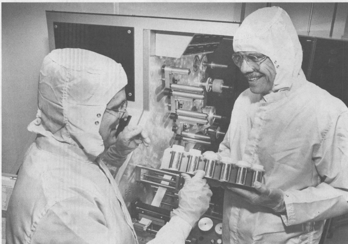
MICHAEL MCDONALD (7484, left) and Bill Alzheimer (7400) examine parts made on the computer-controlled CL805 capacitor winding machine. The CL805 is featured in the first issue of Manufacturing Technology , the first of three quarterly bulletins published by Sandia to stimulate industrial interest in technology transfer activities at the Labs. Bill is technical consultant for Manufacturing Technology .
