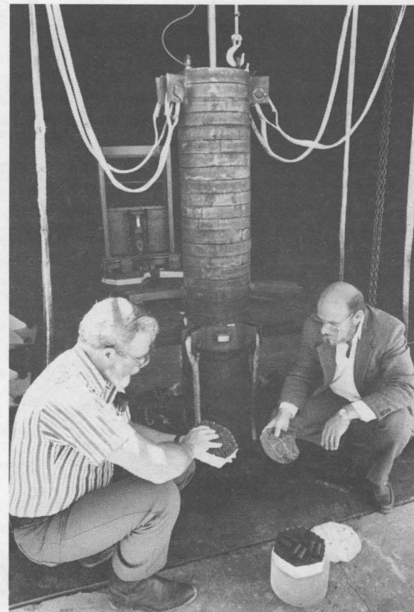
DROP TEST SETUP is checked out by Karl Schuler (left, 1544) and Paul Cooper (9333). The cylindrical stack behind them is formed by weights that determine the energy of impact.
