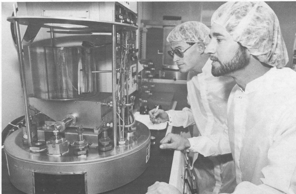
"GROWING" SUPERCONDUCTING thin films on a substrate with an electron-beam evaporator are Tom Zipperian (back) and Thomas Plut (both 1141).
