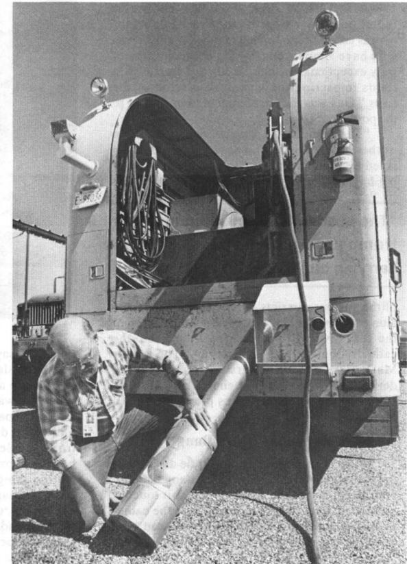
DON SHADEL (9331) has developed a series of TV cameras for downhole viewing. The 80-pound camera Don is displaying was, he says, "conceived, designed, and built" by Sandia at NTS. Other models fit inside vertical holes as small as 4 inches in diameter.
