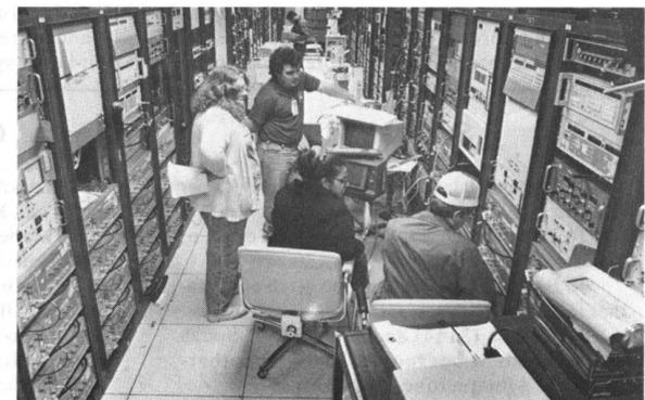
COLLECTION OF DATA from tests is the purpose of this room, staffed by employees of EG&G under technical supervision by Sandia. Most data is now carried out the entrance of the tunnel by fiber optic cables and transmitted several miles for central collection. Formerly, it went vertically through drill-holes to the mesa top for recording on equipment housed in trailers.
