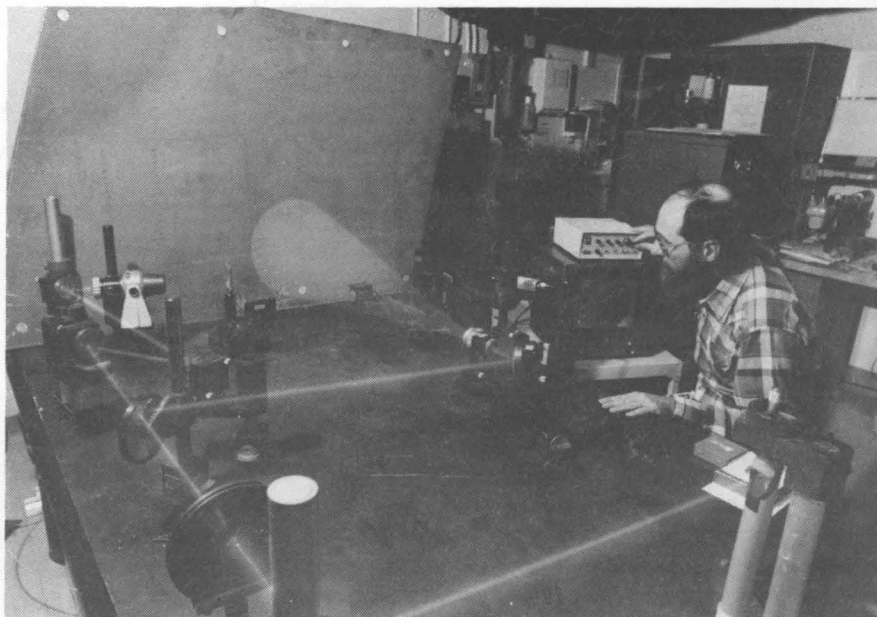
BRUCE HANSCH (7551) uses laser interferometry to inspect a section of an aluminum aircraft wing. When the wing surface is stressed with vibration, heat, or pressure, flaws manifest themselves by causing larger displacements of the laser beam.
