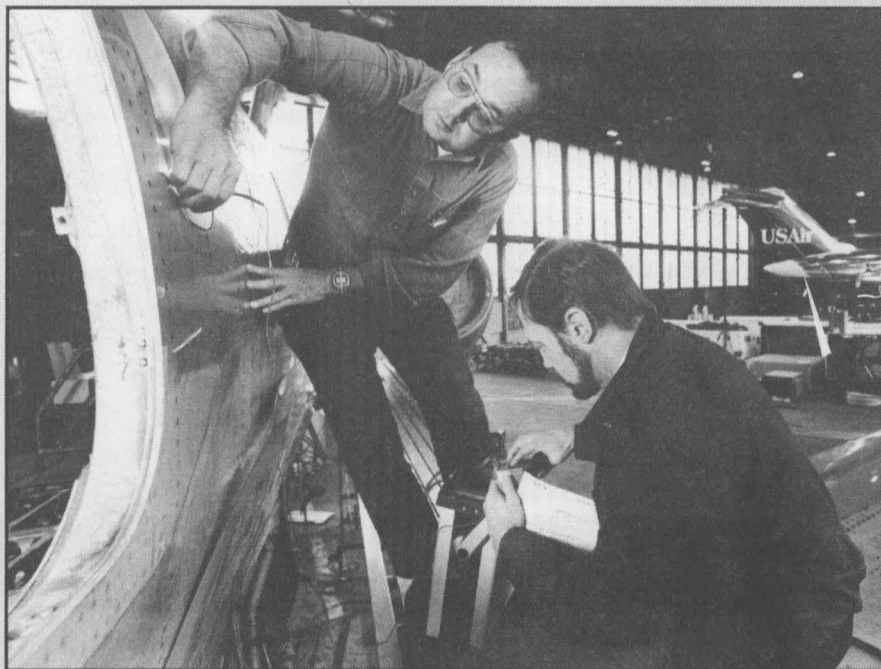
LOOKING FOR FLAWS — USAir employees apply an eddy current device to detect flaws that cannot be seen by the naked eye. (Photo courtesy USAir)
