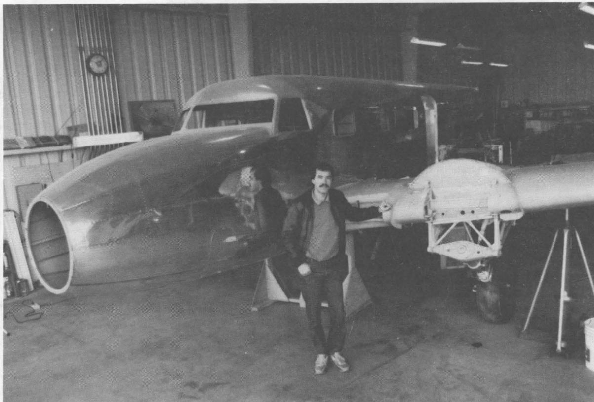
STANDING NEXT to the partially finished body of his Lockheed 12A is Yon Perras (8441). The plane when fully restored will be 36 feet, 4 inches long from nose to tail, with a wingspan of 49 feet, 6 inches. Overall weight of the eight-passenger aircraft is 8,750 pounds, lighter than normal due to its all-aluminum construction.
