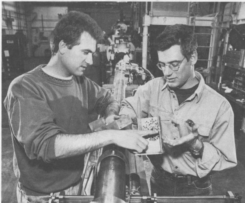
CHECKING RESULTS — Herbert Negele (left) and Jurgen Srnik examine results after fragments from a hypervelocity impact struck a piece of metal. They and two fellow Technical University of Munich graduate engineering students performed experimental work during a two-month stay at Sandia.
