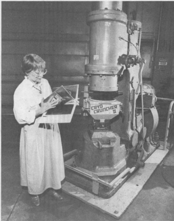
PIECE-WORK MACHINE — Pat Neiswander of Weapons Waste Management Technology Dept. 6623 looks through photos of examples of the tiny pieces of material left after a weapon component is cryofractured. Pat says those familiar with the forge hammer nicknamed "Cryo Cruncher II" have coined a word for the process in which it smashes components made brittle by a bath in liquid nitrogen — "rubble-izing."
