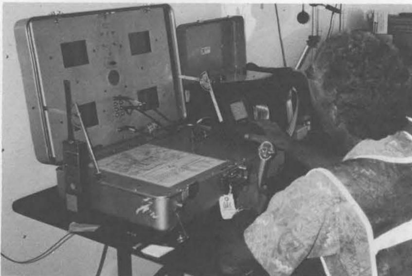
DAVE SHIREY (9567) operates the Portable Integrated Video System during a field exercise. The hand-carried system, packaged in suitcases, would transmit video and audio information as well as computer data over a single fiber-optic cable from the site of a nuclear accident to a command post.
