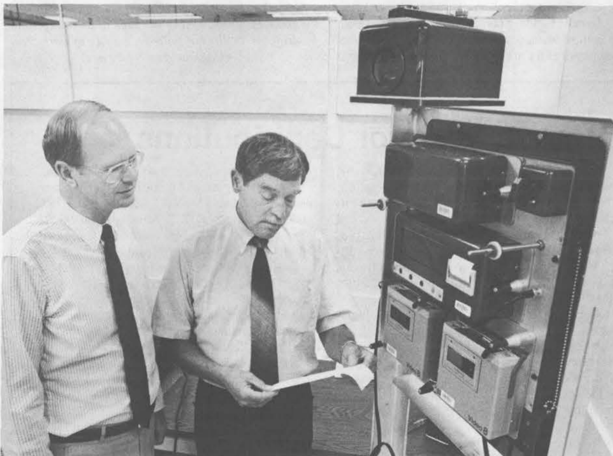
PROTECTING NUCLEAR MATERIAL — Duane Landa (7180, left) and Dennis Mangan (9249) look at a Sandia-designed Modular Integrated Video System (MIVS). To ensure that nuclear material is being used for peaceful purposes only, the MIVS is used for surveillance at sites monitored by the International Atomic Energy Agency (IAEA). Duane has worked to have the US government provide for easier export of safeguards equipment such as this. MIVS is manufactured by an Albuquerque firm, Aquila Technologies; about 200 units have been or will be installed worldwide. Other Sandia-designed safeguards and security hardware includes the Cobra fiber-optic seal, in use by the IAEA and EURATOM; information authentication monitoring systems installed in two facilities in Japan; and (in a collaborative project with Los Alamos National Lab) a system that combines radiation detectors with video surveillance, installed in the United Kingdom. The two latter systems are undergoing field tests.
