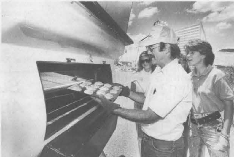
THE VILLAGER — Patricia Cordeiro (6215, right) and Phyllis Best watch Lindsey Evans (both contractors) remove cookies from a Burns-Milwaukee Villager Sun Oven being tested at Sandia. This oven can bake up to 50 loaves of bread in an hour. It may be used to help feed large groups in areas where conventional power isn't available.
