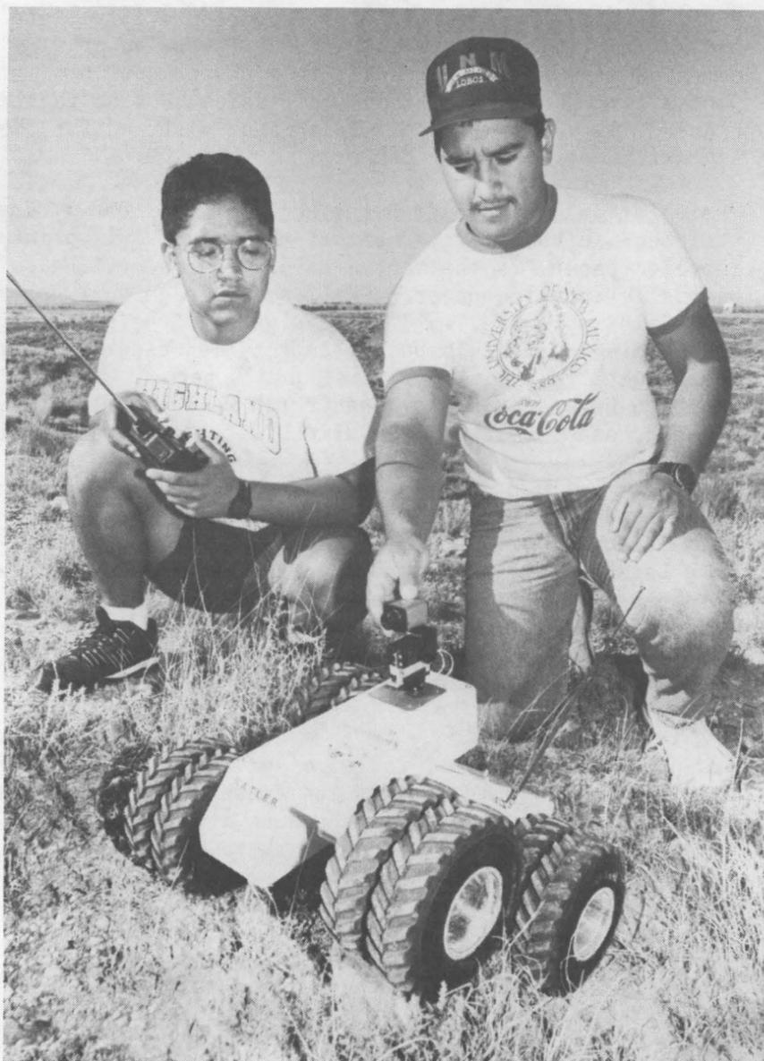
THIS RATLER DOESN'T BITE — Students Leon Martine (left) and Adan Delgado (both 9616) prepare to put a model of Sandia's Robotic All-Terrain Lunar Exploration Rover (RATLER) through its paces traversing rugged rocks and hills around Sandia's Robotic Vehicle Range. RATLER is Sandia's first of a new breed of space robots known as micro-rovers designed to have a small launch mass and yet large payload capacity. (Photo by Randy Montoya)
