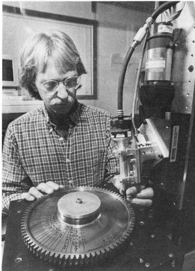
HISTORY IN FLEXIBLE MANUFACTURING — Two years ago, Sandia helped Pratt & Whitney develop this robotic deburring system that automatically grinds edges of jet engine turbine wheels during manufacture. The system uses computer-aided design (CAD) models and computer vision and force control sensors to match the part to precise specifications. Cliff Loucks (1611) and Colin Selleck (1661, not seen) developed the system. (LAB NEWS, March 9, 1990)
