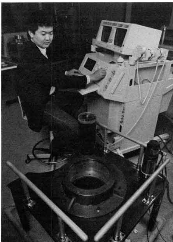
ALAN MORIMOTO (1671) at the controls of an ultrasonic scanner used in a computerized scanning technique developed at Sandia. It can create a three-dimensional map of the residual limbs of amputees showing the precise locations of skin surfaces and bones. Such information can be used for fabricating prosthetic devices. Sandia is working with the University of Texas Health Science Center at San Antonio to develop the technology. This is one of several biomedical engineering projects now under way at Sandia.
