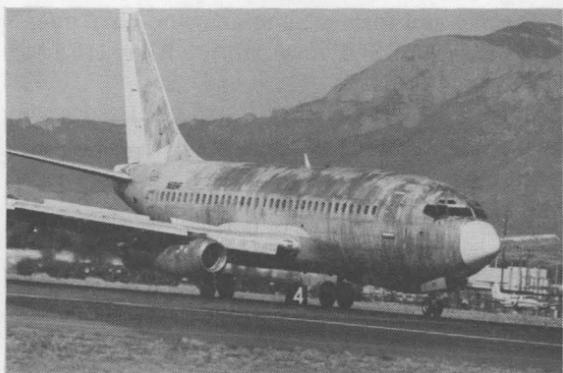
WORSE FOR WEAR — An over-the-hill 737 transport plane lands at Albuquerque. It's now used for research on inspecting aging aircraft.
