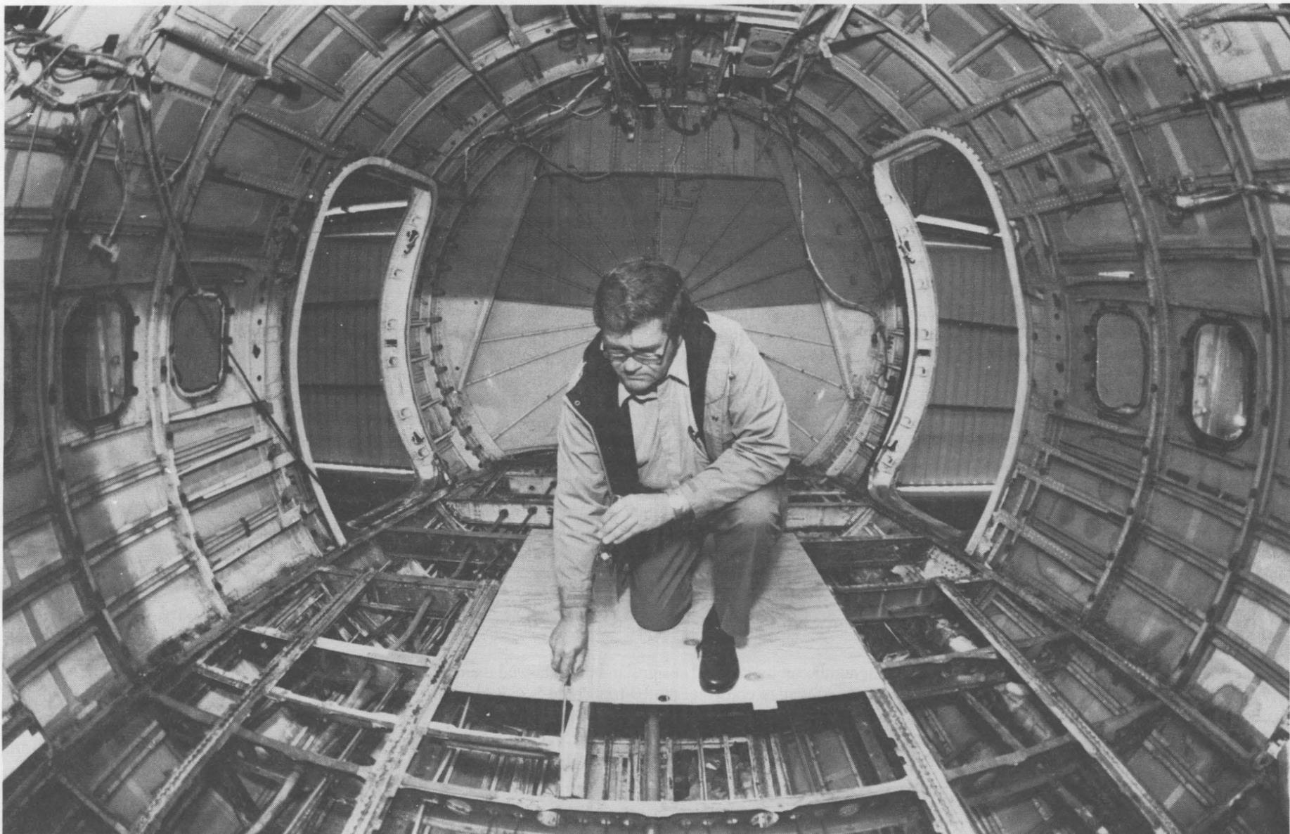
HOLLOW SHELL — Ken Harmon of Aerodynamics Dept. 1554 examines the interior of a 737 transport plane to be used as part of Aging Aircraft Non-destructive Inspection Validation Center research at Sandia. (Photos by Randy Montoya)
