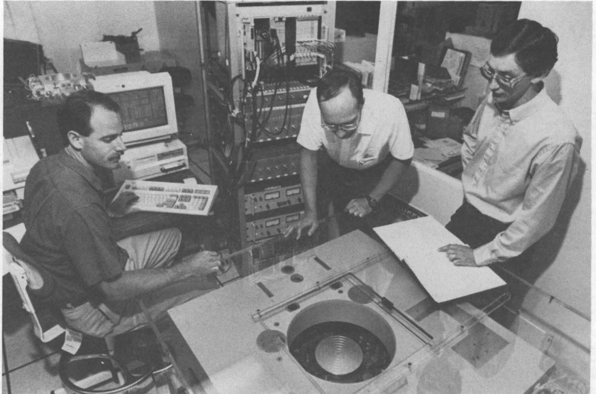
**FLOATING BY MAGNETISM:** From left, Doug Jordan, Joel Darnold, and John Wronosky (all of Manufacturing Applications Dept. 2338) are part of a team developing this magnetically levitated positioner. The technology could be used for ultra-precision applications such as integrated-circuit manufacturing.
