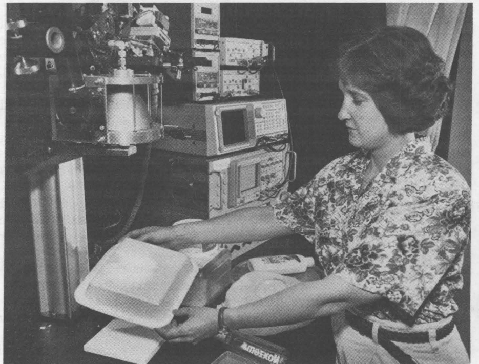
HOLDING a plastic foam food container up to a near-infrared light source, Suzanne Stanton (2338) demonstrates an automatic sorting technology developed at Sandia that can identify various types of plastics right on a recycling plant conveyor belt. The approach combines spectroscopic techniques with a computer neural network "trained" to recognize distinct spectral patterns given off when light is reflected off plastic surfaces. And it works at a speed of about 13 containers per second.
