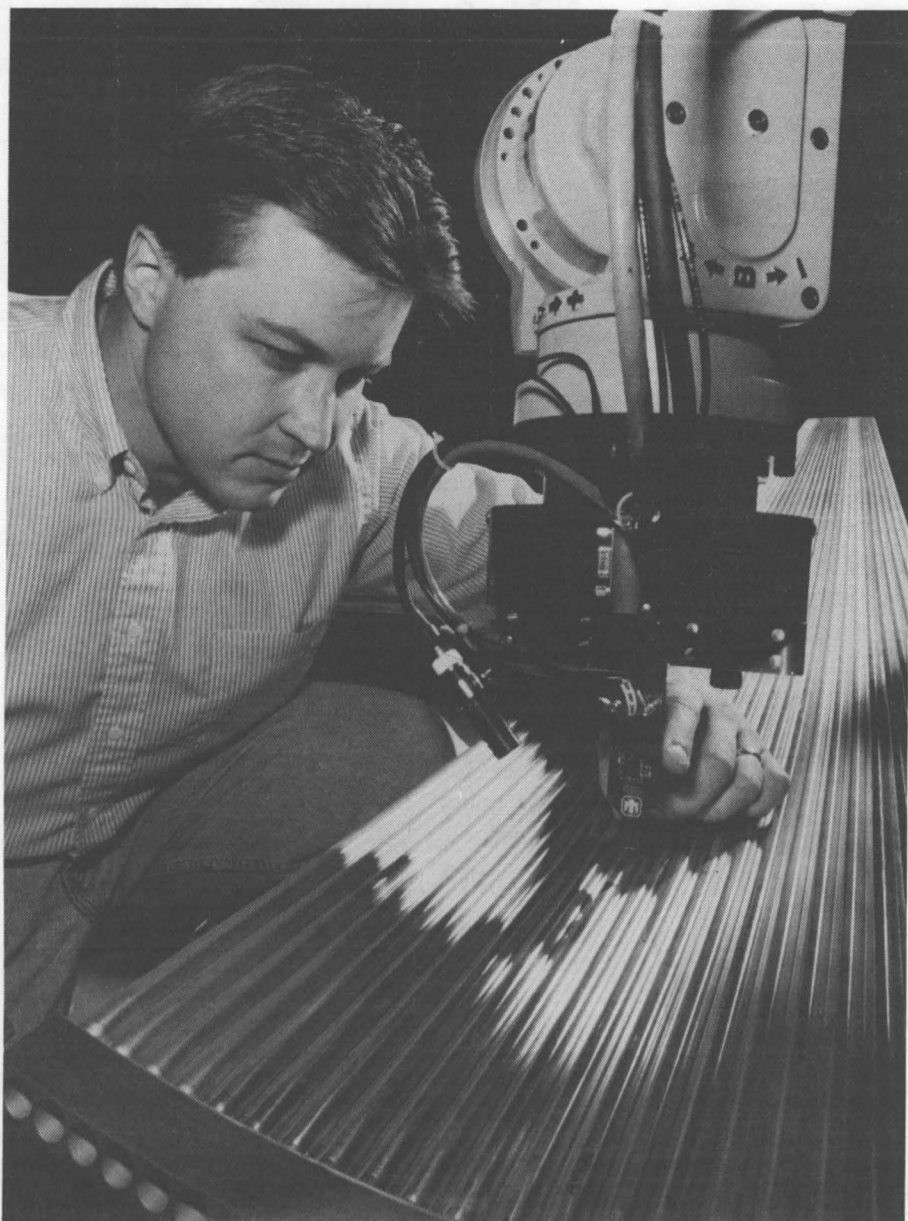
JIM NOVAK (1611) adjusts a Sandia-developed sensor system that will speed the brazing of tubes for a rocket engine thrust chamber and save material costs as well. (Photo by Mark Poulsen)
