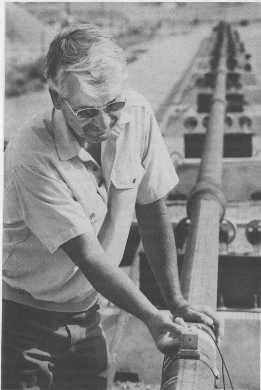
ORPHEUS RANGE — Doug Drumheller (6111) checks an accelerometer used to measure motion along 1,500 feet of steel drilling pipe at Orpheus Range in Tech Area 3. The horizontally mounted pipe at the range is being used for a number of drilling projects, including efforts to improve transmission of data by sound waves from deep within a well. (Photo by Randy Montoya)
