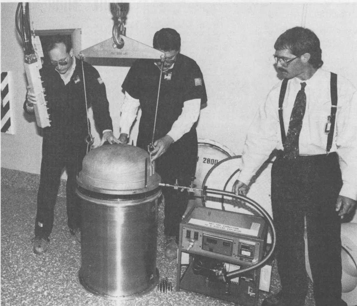
A NUCLEAR WEAPON PARTS shipping container is displayed and explained at a recent "media day" at DOE's Pantex nuclear weapon assembly/disassembly plant in Amarillo, Texas. These Pantex employees — (from left) Jerry Ithaca, Randy Twombly, and Gary Cockrell — demonstrated how the nearly indestructible container is checked to ensure that it is completely leak-tight before any parts go into it for shipping. DOE showed more than 30 print and broadcast people many parts of the Pantex plant that had never before been seen by the public. Sandia has offices and employees at Pantex and is working with the plant to help design weapon dismantlement technology that better ensures worker and environmental safety. The LAB NEWS will soon feature this work.
