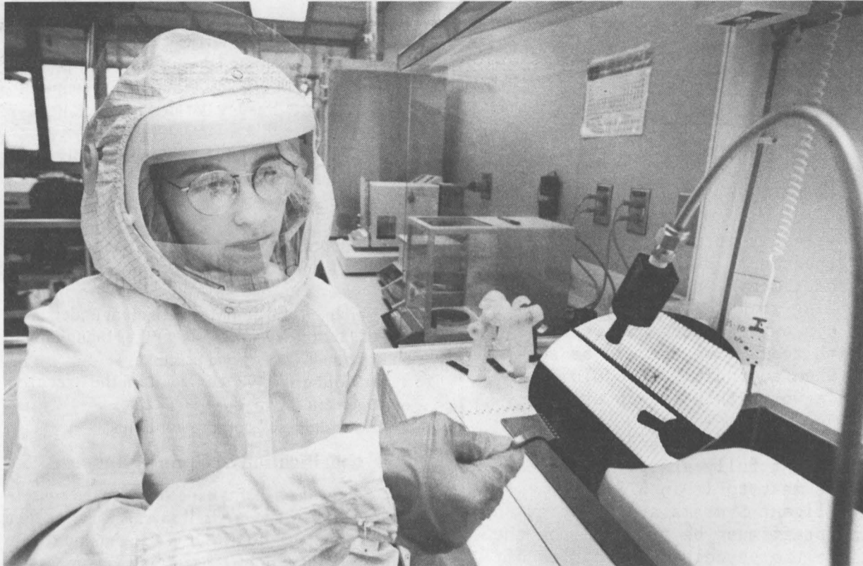
TRICKY CONTAMINANTS — Nicole Korbe of Films and Operations Dept. 1323 artificially contaminates a silicon wafer by spraying silicon nitride particles onto its surface. Once contaminated, the wafer will be subjected to advanced cleaning techniques being developed at Sandia's Contamination-Free Manufacturing Research Center. (Photo by Randy Montoya)
