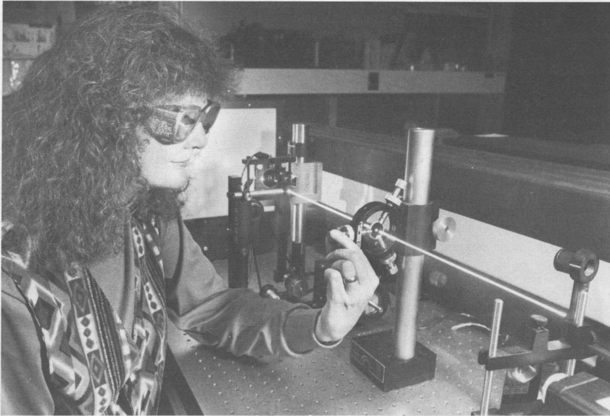
JUDY ODINEK (1153) adjusts laser equipment as part of an experiment to study a unique family of substances called electrorheological fluids that transform from liquid to solid in the presence of an electric field. In the experiment, laser light scatters as it passes through a transparent fluid. The resulting pattern of light appearing on the screen behind Judy tells researchers how the fluids' structures flow and break up under stress. (Photo by Randy Montoya)
