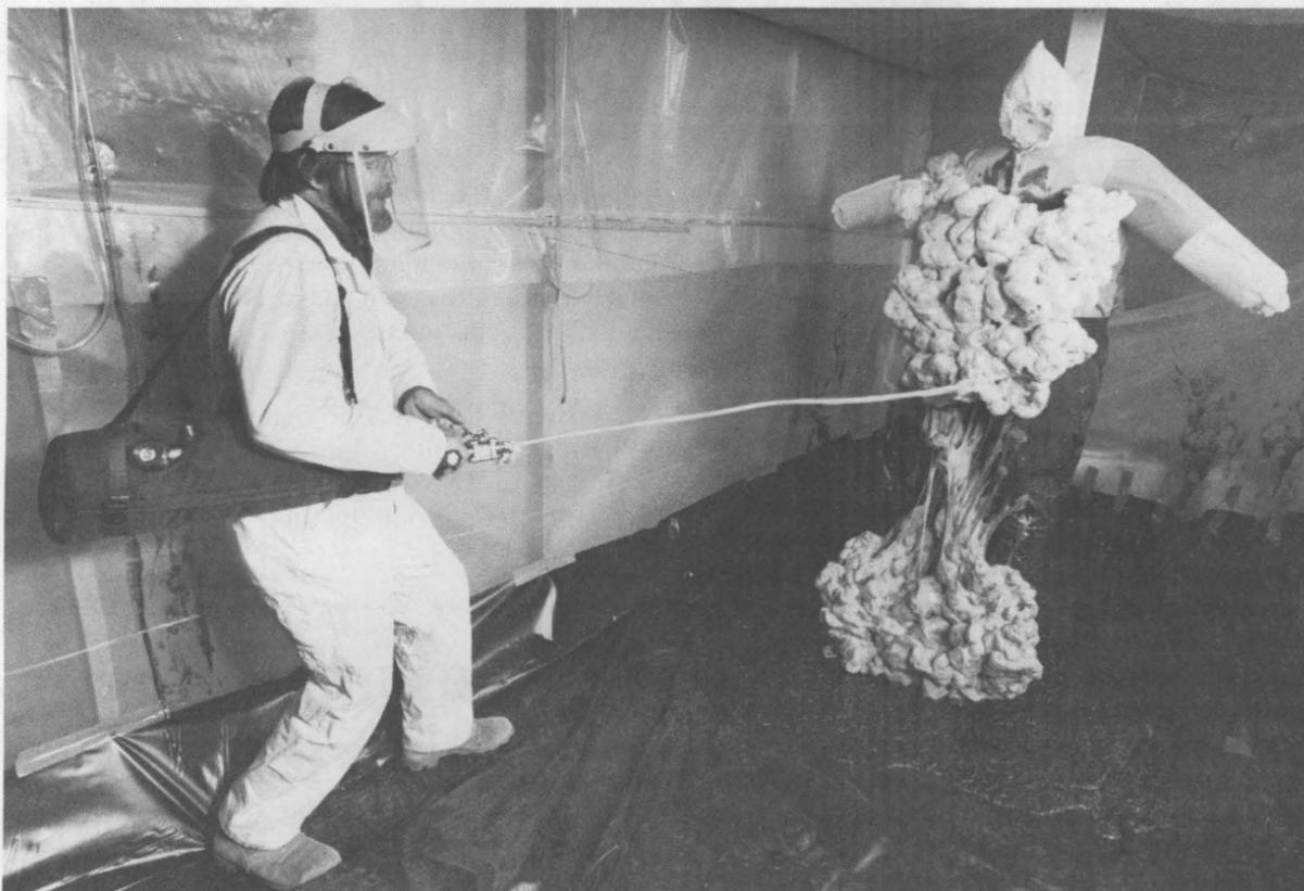
FOAM FOR FELONS — Jeff McDowell of Access Delay Technology Dept. 9611 sprays a mannequin with sticky foam using a new sticky foam gun he built and helped test. The gun is among a relatively new class of "less-than-lethal" weapons for law enforcement that temporarily disable, rather than kill, their human targets. It is likely to get its first use in US prisons. (Photo by Randy Montoya)
