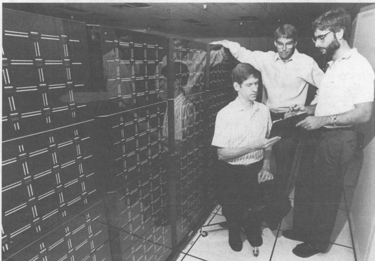
RECORD BREAKERS — David Womble (1422, seated), Art Hale (1424, middle), and David Greenberg (1423) examine data documenting the world-record LINPACK benchmark speed of 143.4 gigaflops achieved on Sandia's Intel XP/S 140 massively parallel supercomputer. Four of the computer's more than 30 modules are visible. Stephen Wheat (1424) and Intel scientists Greg Henry, Satya Gupta, and Jerry Baugh also were part of the team that broke the world record for computing performance. (Photo by Mark Poulsen)
