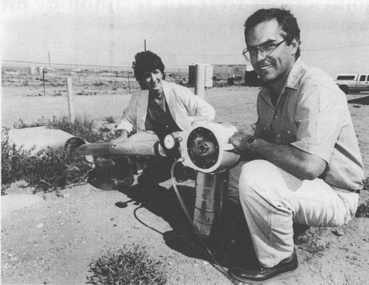
**REVOLUTIONARY SAMPLER** — Cecelia Williams of Environmental Restoration Technologies Dept. 6621 and Bill Lowry of Science and Engineering Associates, Inc., with a demonstration model of the award-winning SEAMIST instrumentation/sampling system they helped develop for sampling fluids and carrying instruments in and out of wellbores quickly. Eastman Cherrington Environmental of Santa Fe is marketing the product for hydrologic studies.
