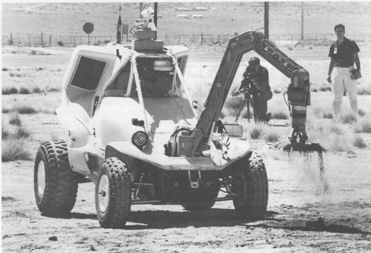
STAR OF THE SHOW — The Remote Telerobotic Vehicle for Intelligent Remediation, or RETRVIR, locates and excavates a buried sign bearing the letters "ISRC" (for Intelligent Systems and Robotics Center 2100) during a recent ground-breaking ceremony for Sandia's new Robotic Manufacturing Science and Engineering Laboratory. (Photo by Randy Montoya)
