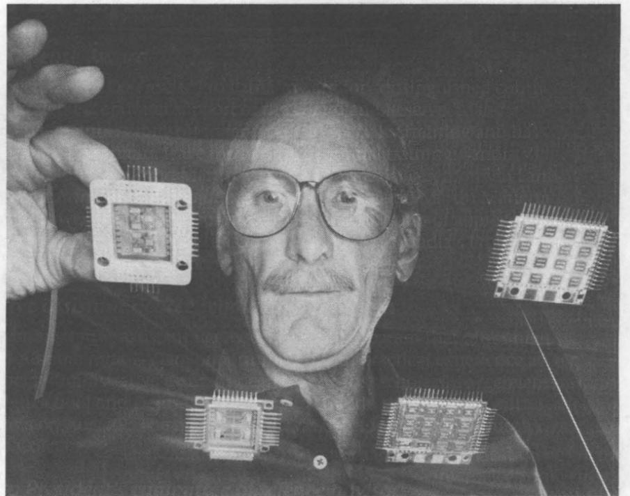
**ELECTRONIC JEWELS** — Don Johnson (contract employee) examines multichip module plates being developed and tested by Sandia. The module's assembly test chips are built on thin diamond substrates that quickly remove heat from the system. Each plate contains 16 chips the size of one square centimeter.
