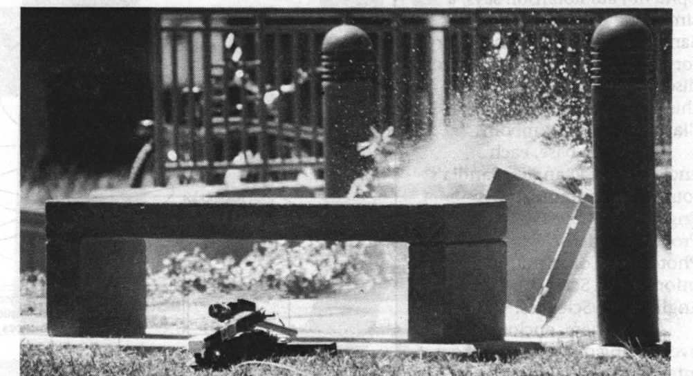
BYE-BYE BOMB — The PAN disrupter blasts a suitcase bomb out from under a park bench at downtown Albuquerque's Civic Plaza, instantaneously disabling the device with a super-high-speed liquid projectile.
