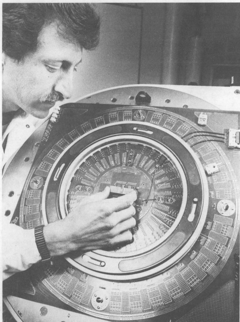
SPEEDY TESTING — Contractor Pat Candelaria conducts quiescent power supply current testing of an integrated circuit at Sandia's Microelectronics Development Laboratory. The instrument enables current testing of integrated circuits at a speed and resolution an order of magnitude beyond previous capabilities. It is capable of performing more than 333,000 current measurements per second, enabling fast, accurate screening of defective circuits. (Photo by Randy Montoya)
