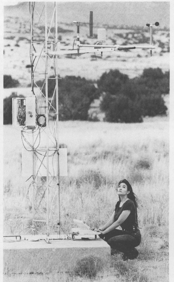
WEATHER REPORT — Danielle Nieto (7575) downloads data from a monitoring station called Schoolhouse Site 1, near the entrance to Coyote Canyon. It is one of nine meteorological/ambient air monitoring stations that make up Sandia's new Clean Air Network.
