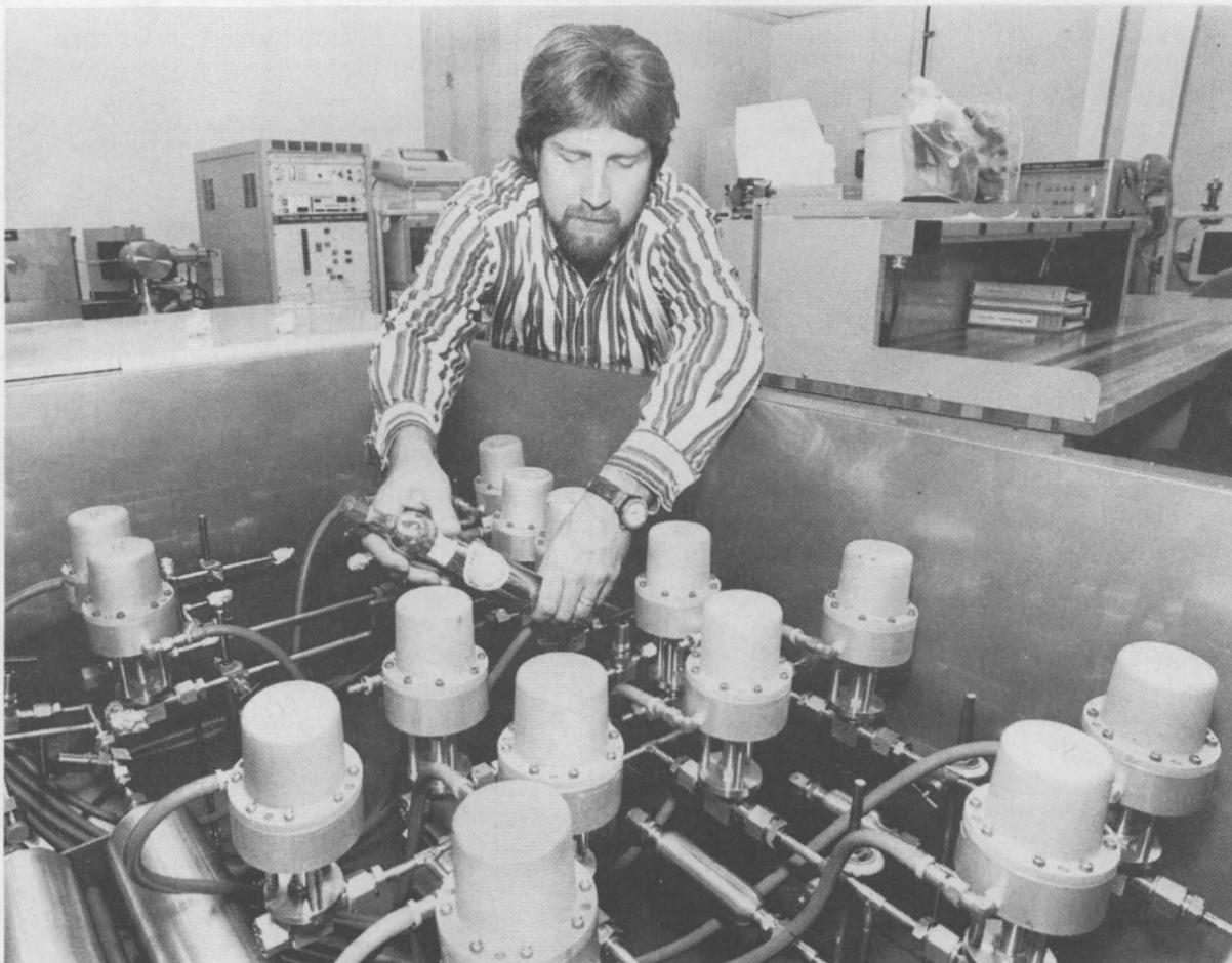
TESTING THE TESTER — Mark Benner (1141) mounts a gas leak standard for testing on the Primary Leak Calibration System array, designed at Sandia. It and other equipment is now available to users from outside DOE's nuclear weapons complex in the just-opened new Primary Standards Laboratory.
