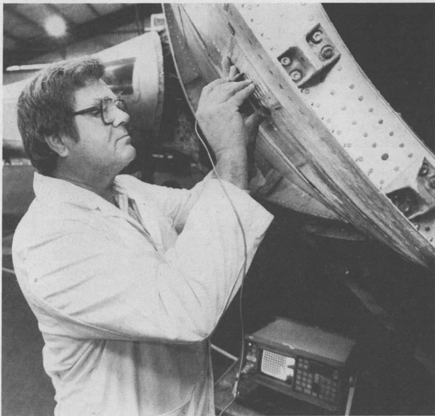
**CHECKING FOR CRACKS** — Ken Harmon, a team supervisor in Sandia's Aging Aircraft Project Dept. 2757, demonstrates the eddy current inspection method on an aircraft fuselage at the Federal Aviation Administration's Aging Aircraft NDI Validation Center, operated by Sandia at Albuquerque International Airport. A Sandia study evaluated the reliability of the method at nine major facilities around the country.
