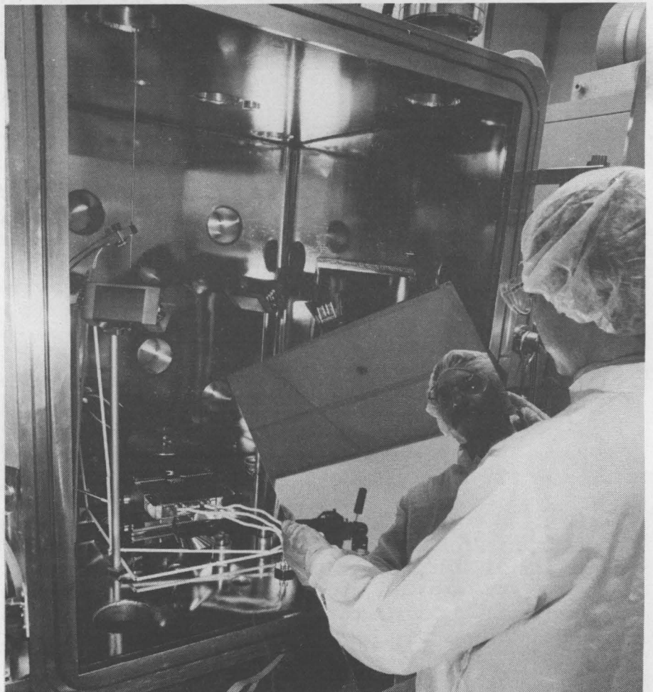
THIN AND FLAT — Juan Romero of Thin Film and Brazing Team 2471-1 examines results of a large-area thin-film test at the National Center for Advanced Information Components Manufacturing, located at Sandia. Large-area thin-film deposition techniques are used in the manufacture of flat-panel displays. Three national labs, eight universities, and 39 companies are involved with the center.
