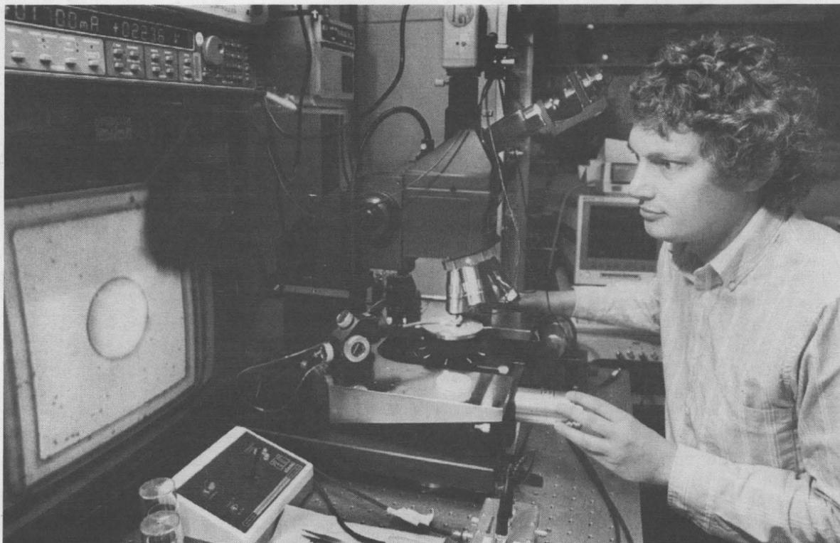
**INNOVATIVE LASER** — Kent Choquette of Photonics Research Dept. 1312 views an enlarged microscopic image on screen of one vertical-cavity surface-emitting laser (VCSEL) out of an array of hundreds.
