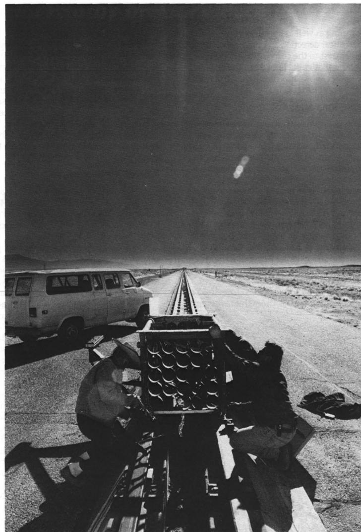
Bolting a sled to the rails in preparation for an acceleration test are (clockwise from left) Bill Kampfe (2761), Dean Jacoby, and Peter Montoya (both contractors). Most sled vehicles are custom designed and built in Sandia's metal shops.
