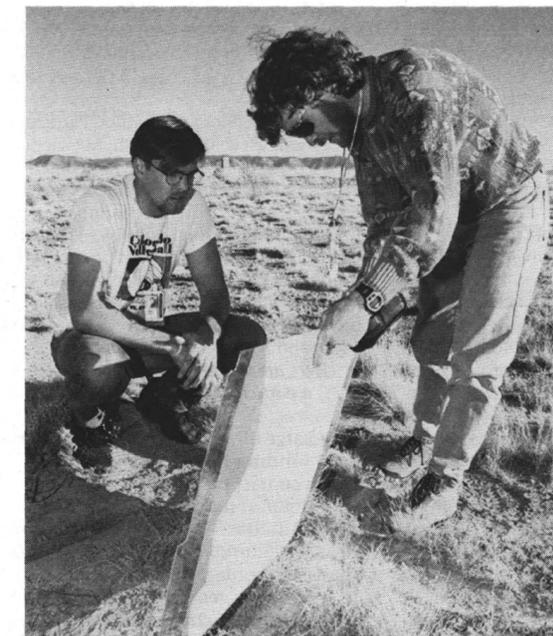
Los Alamos researchers Eric Swenson and Jim Hinckley examine a metal flier plate after it was ejected from a fast-moving sled vehicle at Sandia's sled track facility. The purpose was to test the integrity of material surrounding a spacecraft's power reactor in the event of a launch accident. The test was part of a series of safety tests Los Alamos is sponsoring in preparation for NASA's Cassini exploratory mission to Saturn, scheduled for launch in 1997.
